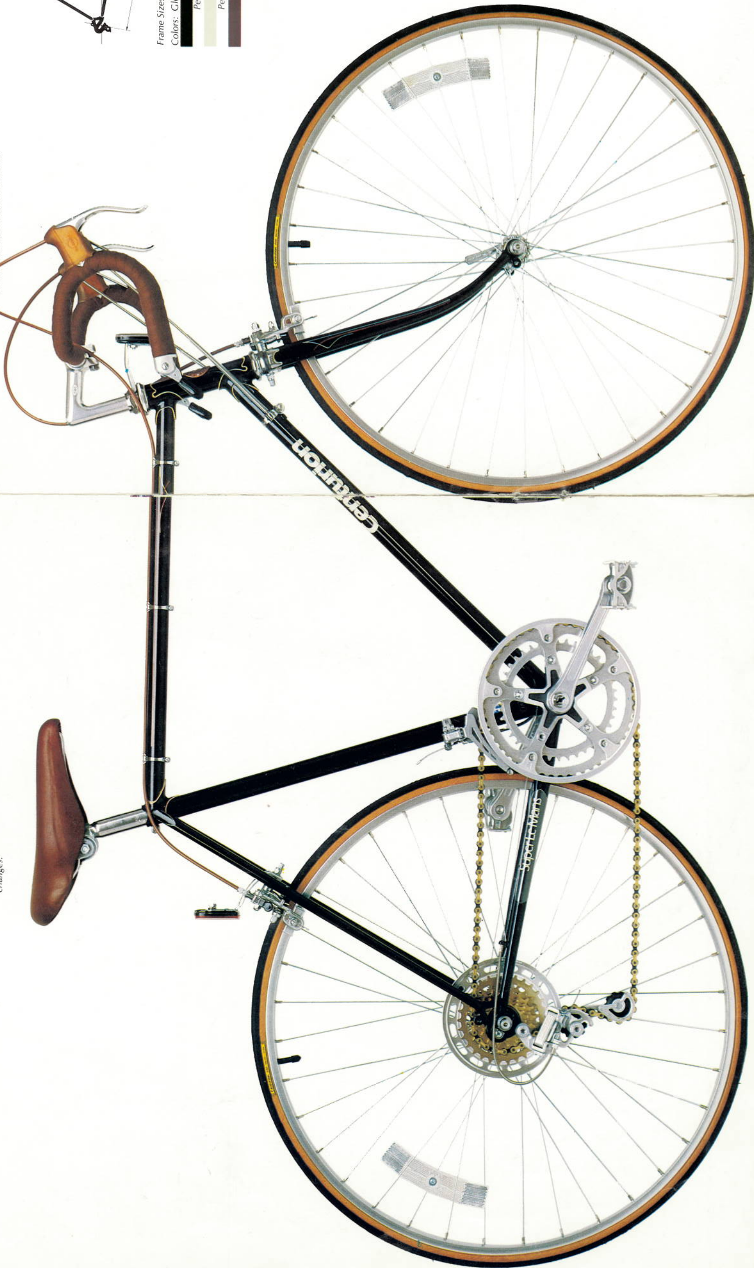
Dia-Compe 500-Q forged alloy side pull brakes with quick release mechanism. Advanced fork design for strength. Chromed crown for racy good looks. Centurion 27" 250 gram 25mm 100 psi skin tires for lightweight roadability.
