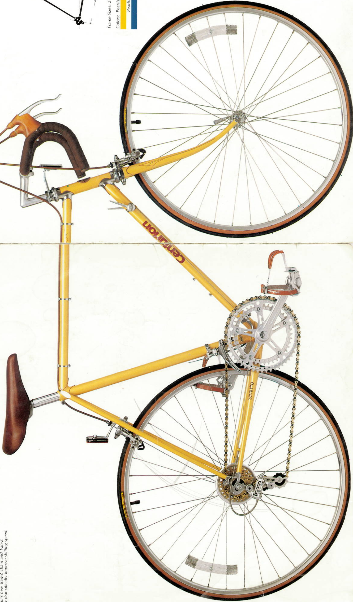
Sugino Super Mighty Victory cotterless forged aircraft alloy crank set, for perfect chain alignment, minimum friction. Forged aluminum pedals with chromoly spindle, and precision bearing races. Toe clips, toe straps. Pro style brazed-on water bottle holder.
