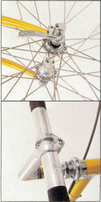
SR New Royal Extra Super Light stem. World Custom engraved handlebar with cloth tape for hand comfort, moisture absorption. Tange professional head set.
