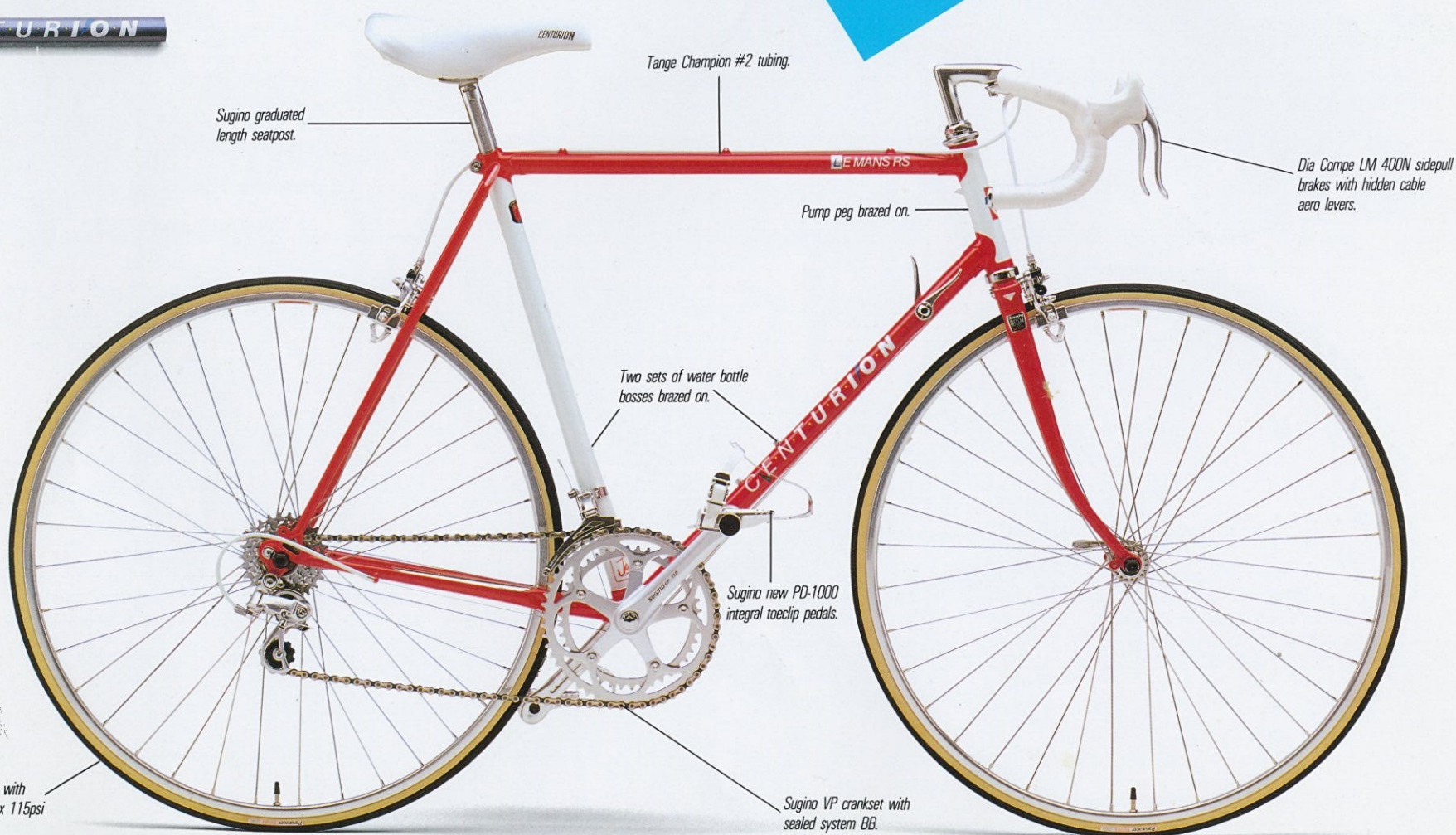
Araya 20C rims with Panaracer Vertex 115psi rated tires. 700C for easy conversion to tubular tires.
