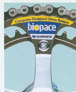
Shimano new 600 EX crank with racing Biopace chainrings.
