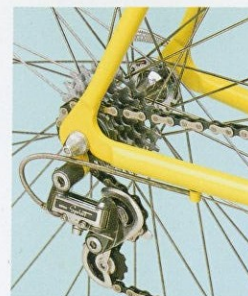
New, Sun Tour Sprint derailleur mounted to specially heat treated aluminum frame drop out.
