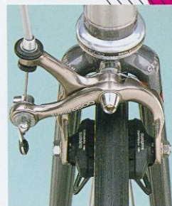
New, composite pads on 600 EX brakes. Special sloping fork crown.
