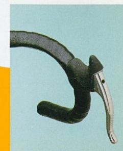
Latest anatomic fit hidden cable aero brake lever.
