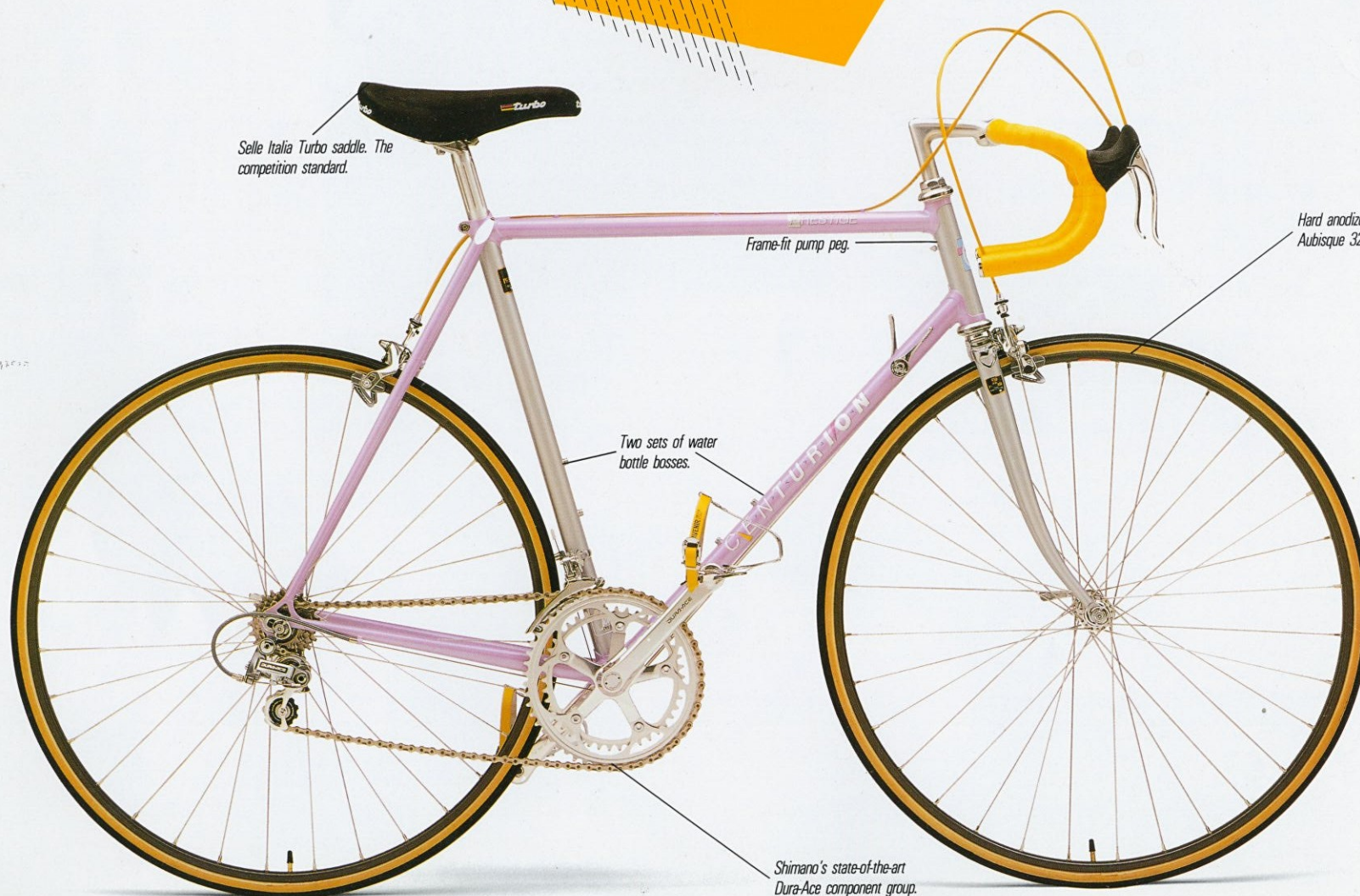
World-class Tange Prestige extra light gauge tubing.
