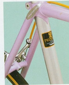
World-class Tange Prestige extra light gauge tubing.
