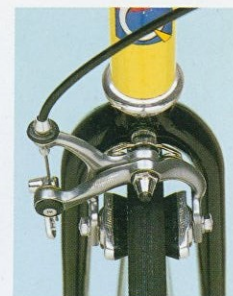
Tange's rigid aluminum alloy Unicrown fork.
