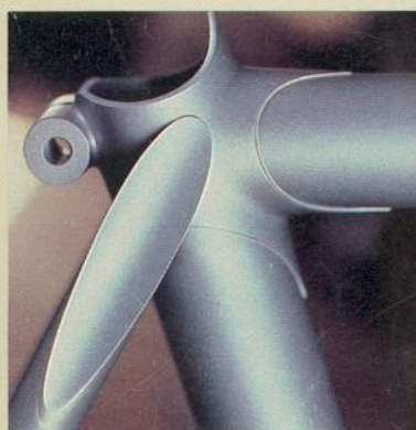
▲ Detail of the fast back seat cluster, a delicate Kellogg design of mitred tubes fitted with absolutely no gaps. Shown here before multiple coats of Dupont Imron® Sable Metallic enamel and clear polyurethane to demonstrate the incredibly clean braising and sanding of the entire "Quest" frame.
