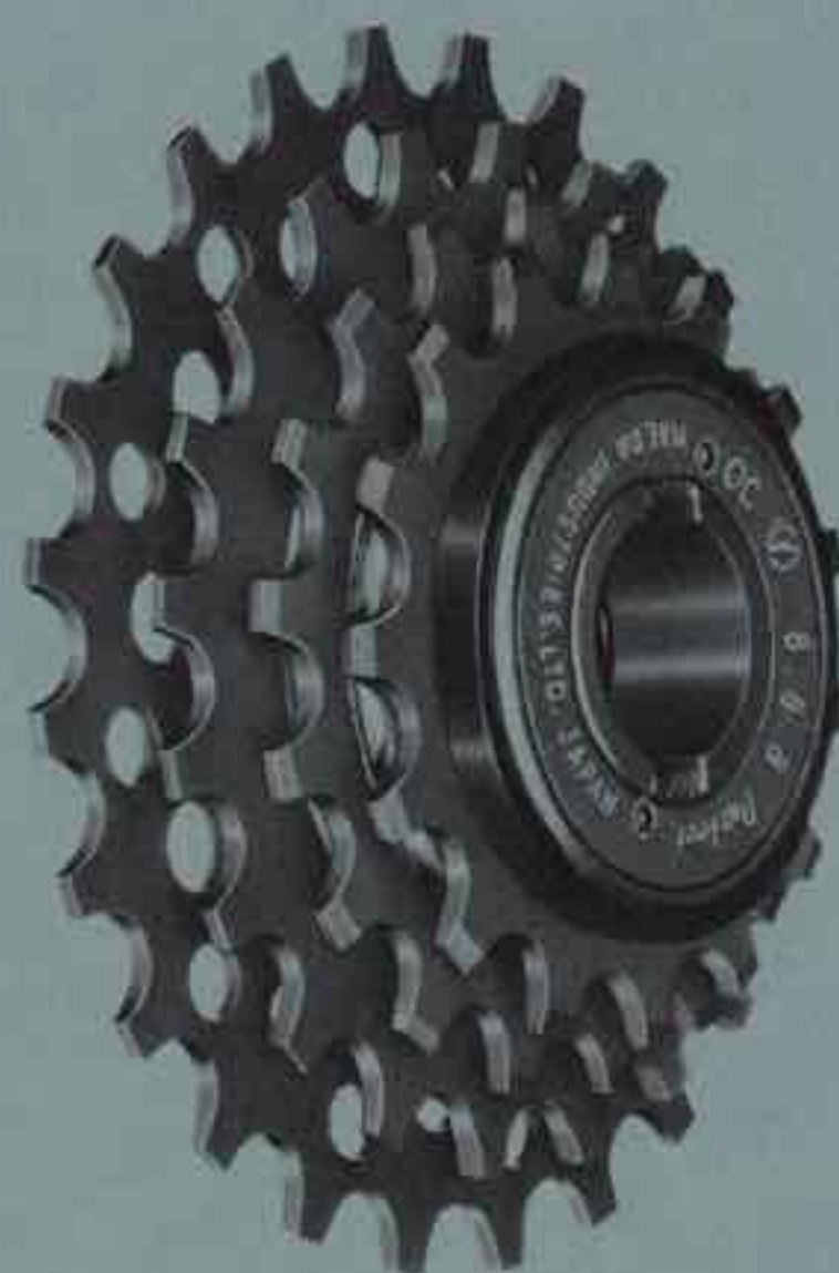
4-SPEED FREEWHEEL No. 1200 Boss type. Brown finish Size: 1/2" x 3/32" x 15, 17, 20 & 24 teeth
