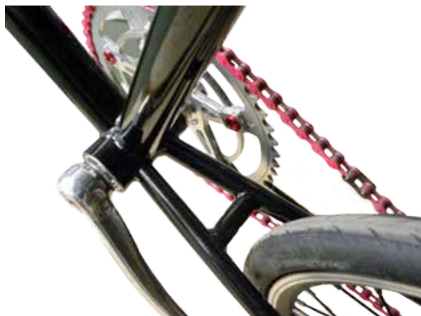
Rear Chain Stay Bridge
