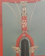
Shimano cantilever mountain brakes offer smooth gradual or instant stopping power.
