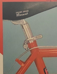
Instantly adjustable quick release seat pillar bolt.
