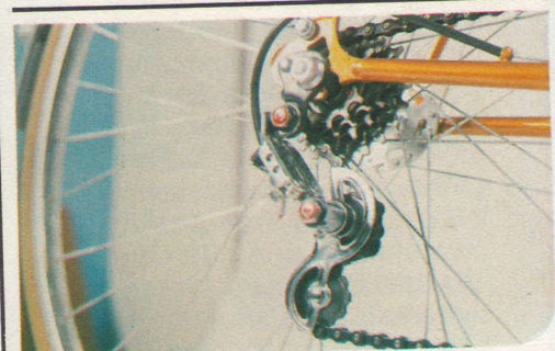
Finely finished rear ends brazed and polished by hand, for strength and appearance
