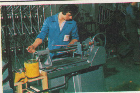
Precision machining to ensure accurate fitting of head and bracket bearings
