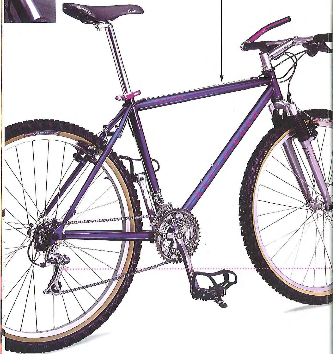
Tange Seiki AheadSet ST-2. Revolutionary way of attaching handlebar stem to the fork. Saves weight while improving the "road feel."
