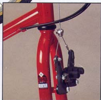
Forks 100% AVR Chromoly. Shimano 201 Cantilever Brakes
