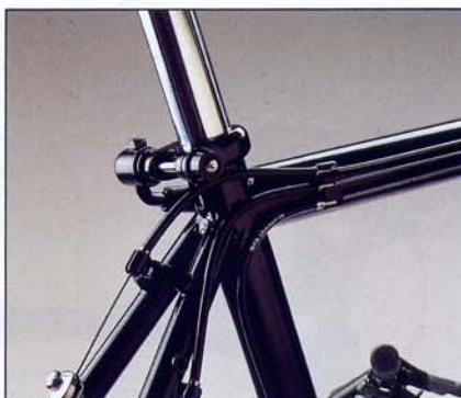
True Temper Double Butted Seat Tube, Cold-Forged Alloy Clamp
