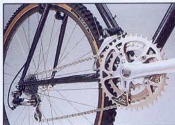
Suntour XC-Pro Micro Drive Crankset 20/32/42T, 11x24T Cassette, and Quick Shifting Short Cage Derailleur
