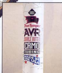
100% Chromoly True Temper AVR Double-Butted main frame
