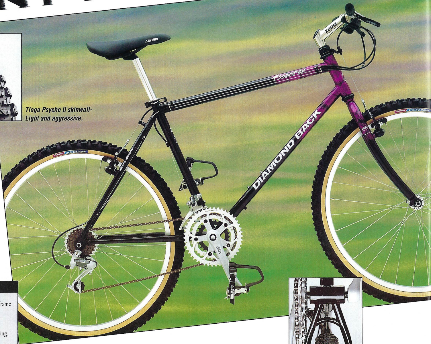
Wider 73mm bottom bracket for increased clearance with even the widest tire.
