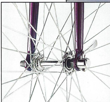
Quick release front hub— Easy wheel removal.
