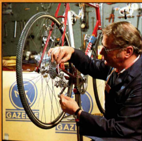
Fitting the operating cable to size and adjusting the rear derailleur.
