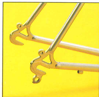
Long model Campagnolo rear ends with mudguard eyes
