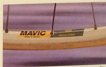
▼ Mavic 195 alloy rims with modified aero profile
