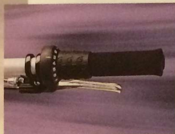
▼ 24-speed Grip Shift SRT-600 shifters
