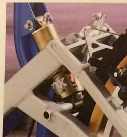
▼ Patented rear suspension shock placement assembly; Custom-tuned Fox rear shock; Easy adjustable preload
