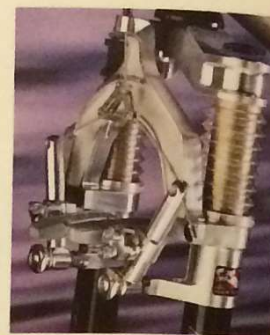
▼ Avid TriAlign brakes with TriDangles and Ti hardware
