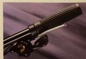
▼ Shimano C-90 Rapid fire TX shifters with optical gear display
