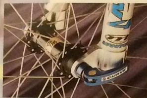
▼ Curve Cycling titanium wheel quick release
