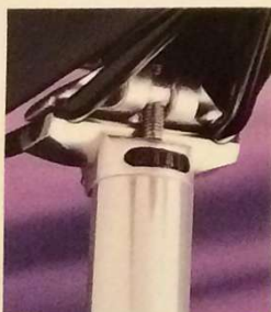
▼ Avenir light alloy seat post with "Dial-Adjust"
