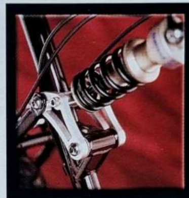
Fastrax Coil-Over Hydraulic-Federelement
