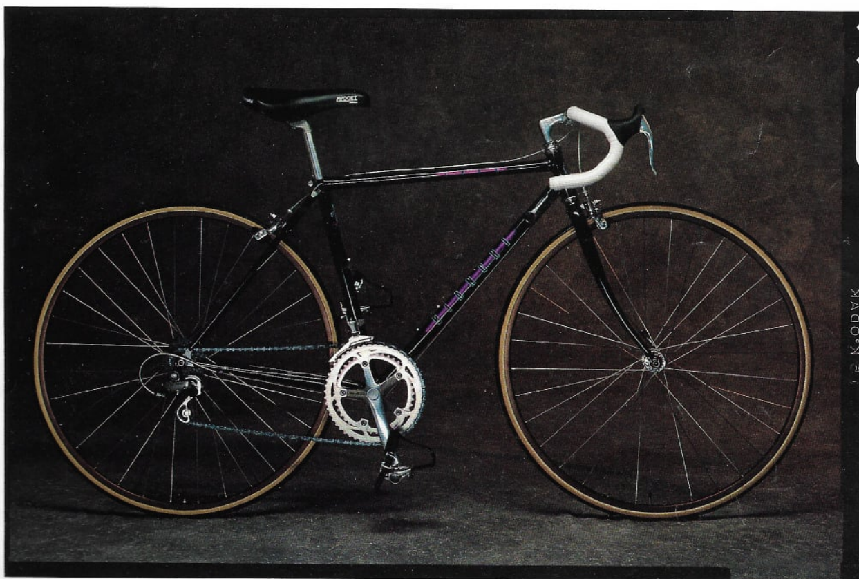
The Bianchi Eros. Simply put, the Eros, a Competition level road bicycle, is a triathlete's dream. With Tange double-buttressed chrome-moly frameset in our SuperSet 2 configuration, SunTour Radius 14-speed component group, Avocet saddle.
