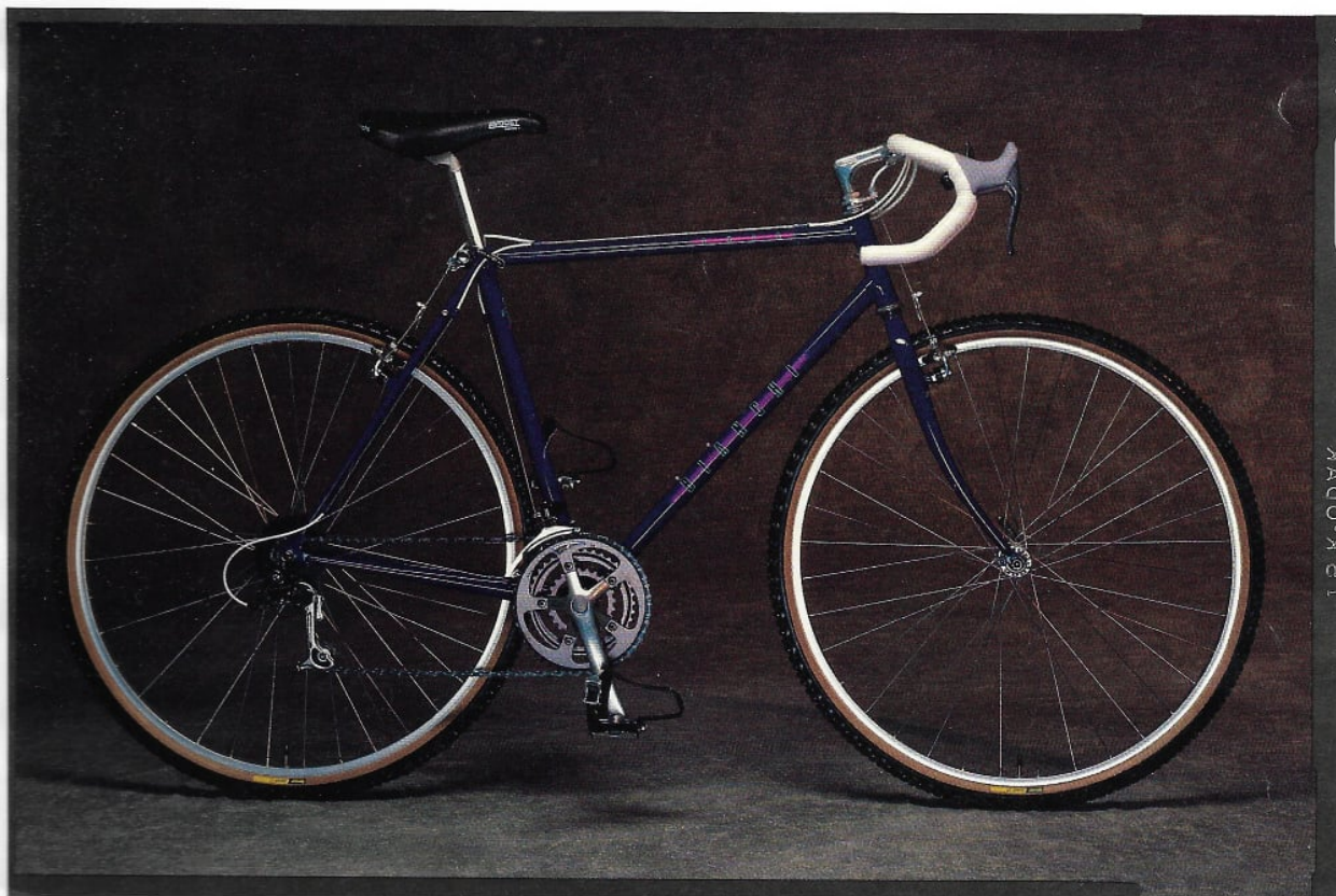
The Bianchi Axis. Built around 38c tires, the Axis offers highly superior off-road capabilities. It's our best Competition level Cross-Terrain bicycle. With Tange double-butt chrome-moly frameset in our SuperSet 2 configuration, Ritchey Force Directional steerer, SunTour XCD 21-speed AccuShift Plus shifting, Araya VX-400 rims.
