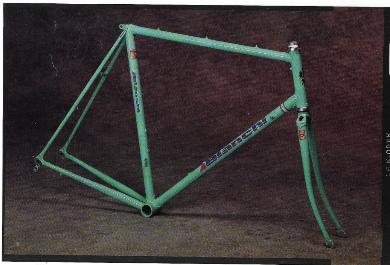
The Mondiale Frameset. The classic Italian road frame built by hand of Columbus SLX/SPX tubing in our SuperSet configuration. With braze on front derailleur mount, investment cast fork crown and seat lug, Bianchi engraving, Cinelli bottom bracket.
