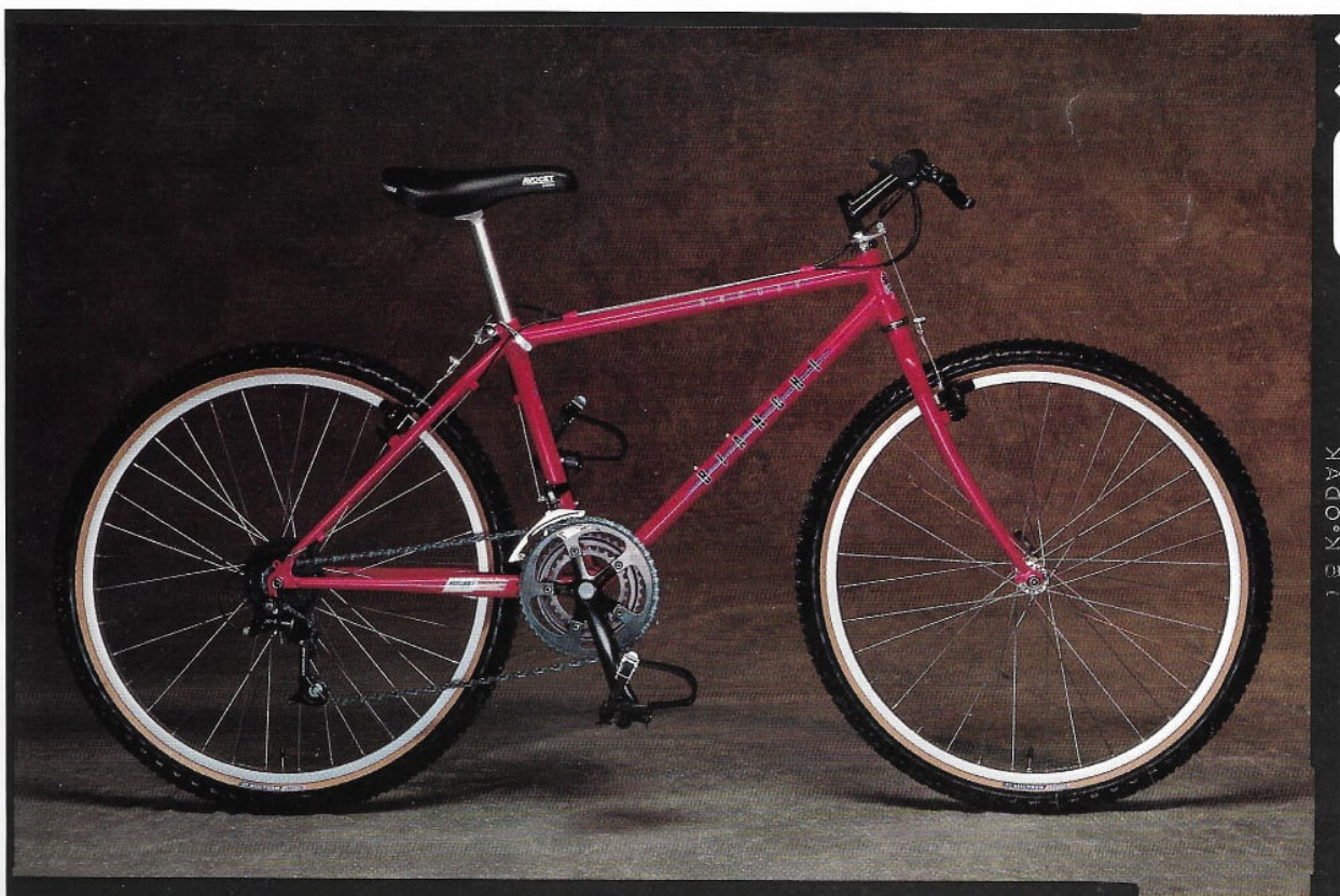
The Bianchi Osprey. The Osprey is a full Competition level Bianchi mountain bike, built around our revolutionary Hi-Wire cabling system. With Tange double-butted chrome-moly frameset in our SuperSet 2 configuration, Ritchey Megabite Overdrive 26x2.0 tires, X-Press shifting, Ritchey Force stem.
