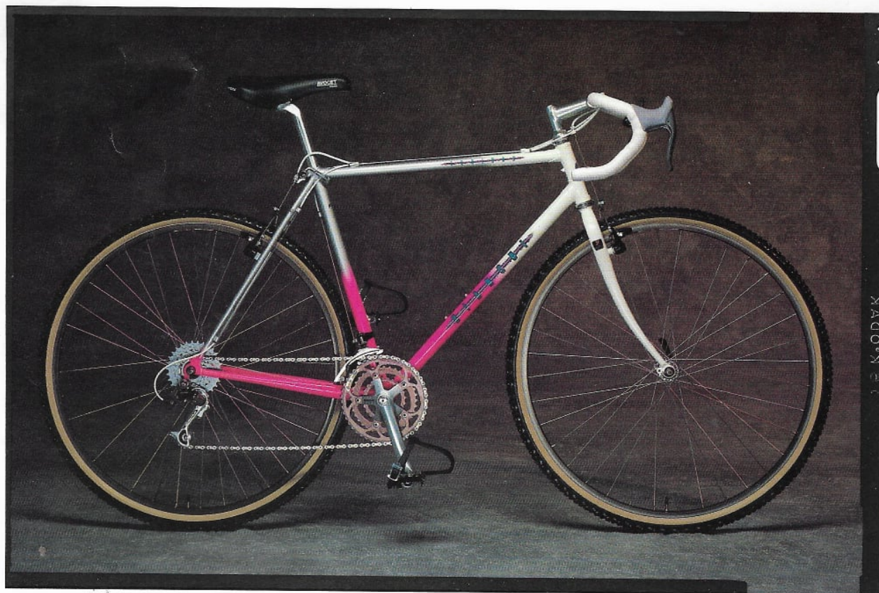
The Bianchi Equinox. Our very best Professional level Cross-Terrain bicycle, representing the state of the art in the most exciting and innovative area in bicycling today. With Tange Prestige frameset in our SuperSet 2 configuration, Ritchey Force Directional Steerer, SunTour XC-Pro 21-speed AccuShift Plus component group, Grease Guard bottom bracket and hubs.
