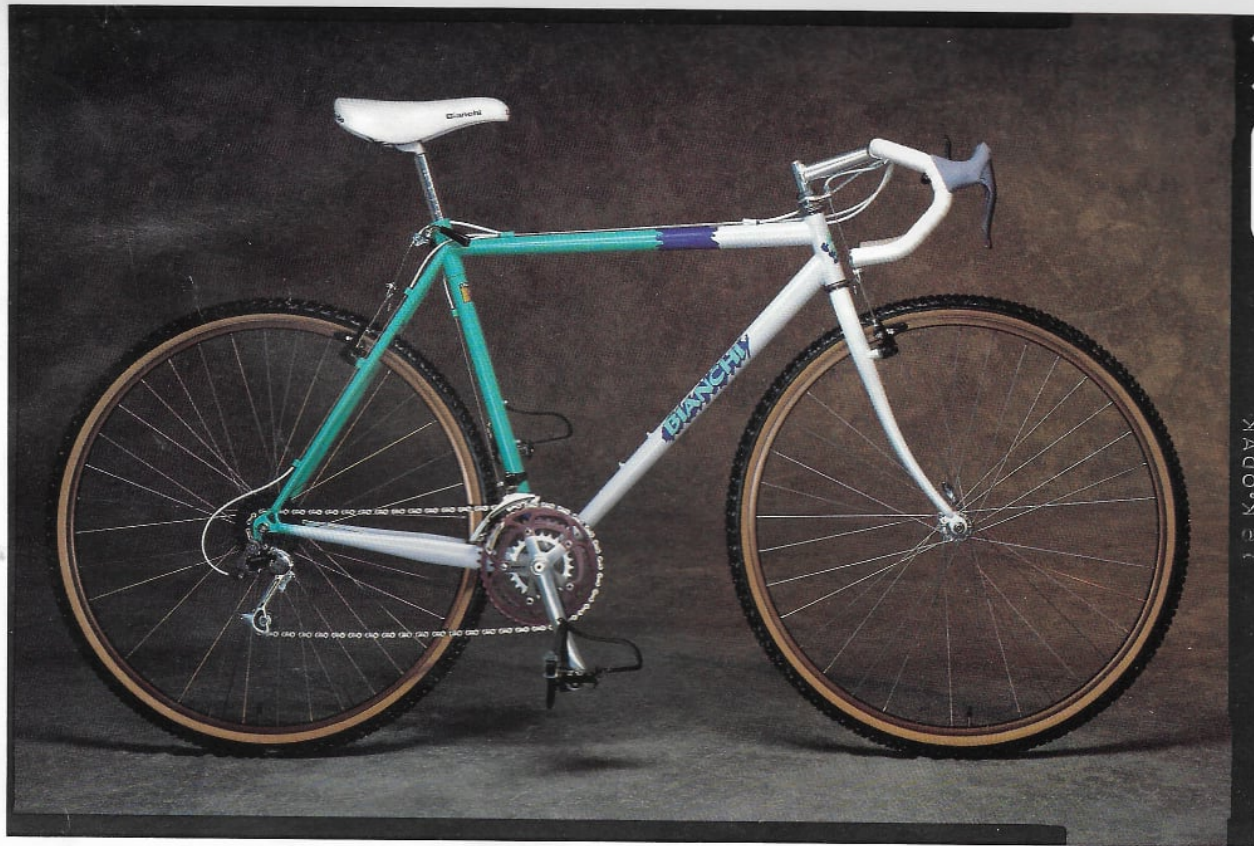
The Bianchi Intercept. Produced in extremely low quantities, the Intercept is the finest Cross-Terrain bicycle we make. With Columbus MAX frameset, SunTour XC-Pro 21-speed AccuShift Plus component group, Command shifters, Grease Guard bottom bracket and hubs.
