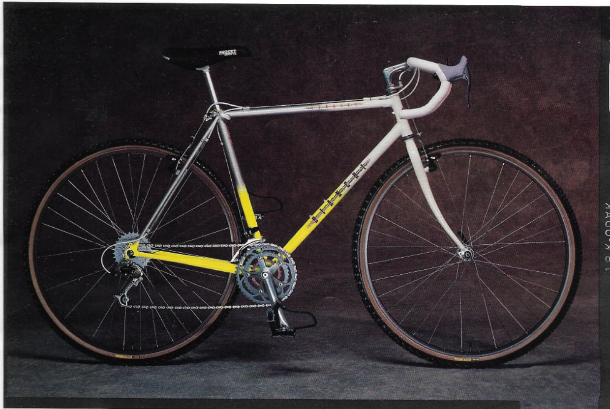
The Bianchi Tangent. A Professional level bicycle, the Tangent offers the road performance of a Cross-Terrain bicycle, coupled with particularly good off-road capabilities. With Tange Prestige frameset in our SuperSet 2 configuration, SunTour XC-Comp 21-speed AccuShift Plus component group, Command shifters, our High-Wire cabling system, Avocet Gelflex saddle.
