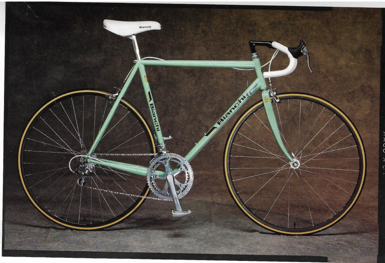
The Bianchi Proto. Entirely hand-fabricated and produced in extremely low volumes, the Proto is the finest road bicycle Bianchi makes. With Columbus MAX frameset, Shimano Dura Ace 16-speed Hyperglide components, Campagnolo Sigma Crono hard anodized rims, Dura Ace clipless pedals.
