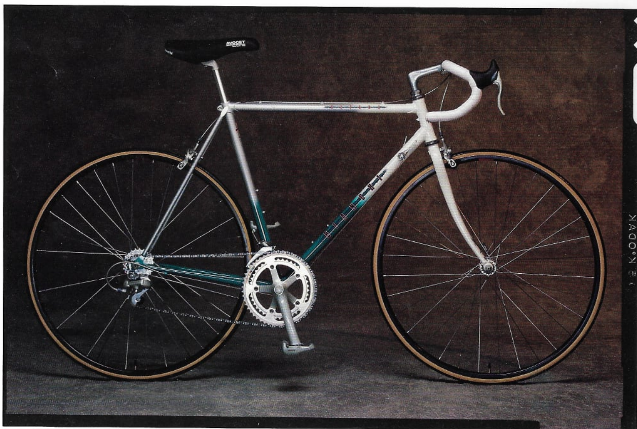
The Bianchi Alfana. Our best Competition level road bicycle, the Alfana is a fully race-ready triathlete's bike offering Prestige tubing in our SuperSet 2 configuration. With Shimano 105 14-speed Hyperglide component group, Shimano 105 clipless pedals, Avocet Gelflex saddle.
