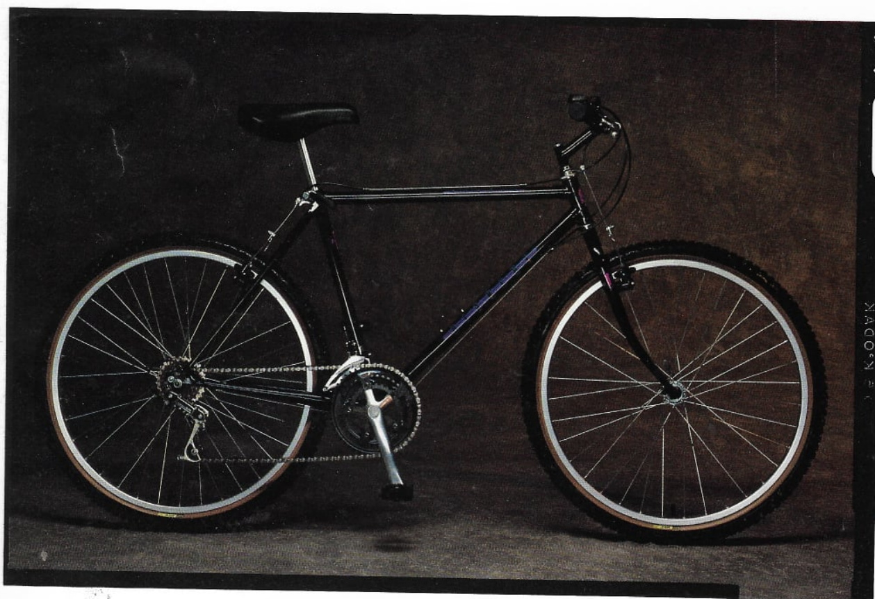
The Bianchi Ocelot. The Ocelot is a full-featured Performance level mountain bike offering rugged, no-compromise 2" tires, and drawing on the venerable Bianchi tradition of design excellence. With Shimano Indexed Hyperglide derailleurs, Bianchi Dakar tires, Araya MP-22 alloy rims, front quick release.
