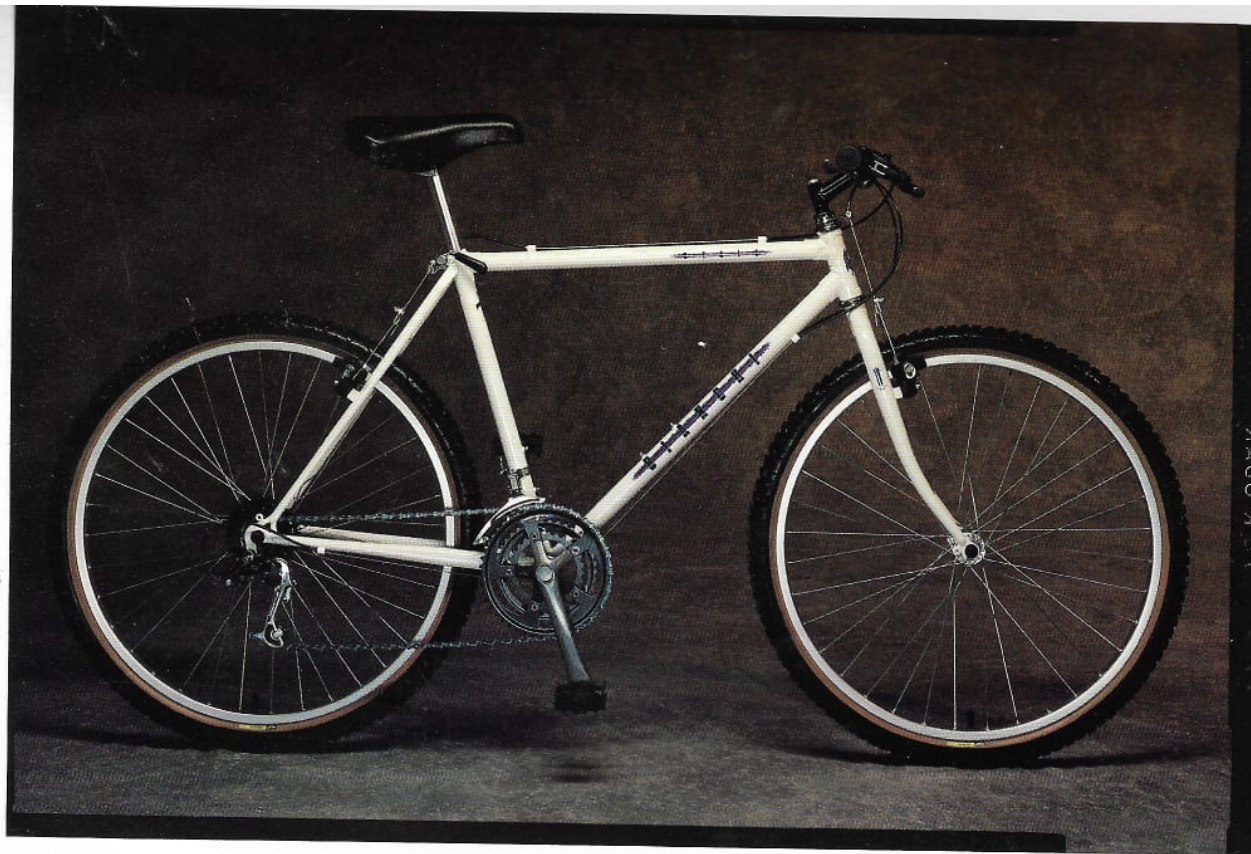
The Bianchi Nyala. Our best Performance level mountain bike, the Nyala is a rugged off-road bike featuring X-Press shifting. With Tange chrome-moly frameset in our SuperSet 2 configuration, SunTour XCT 21-speed AccuShift Plus derailleurs, quick-release hubs, Balance Response brakes.
