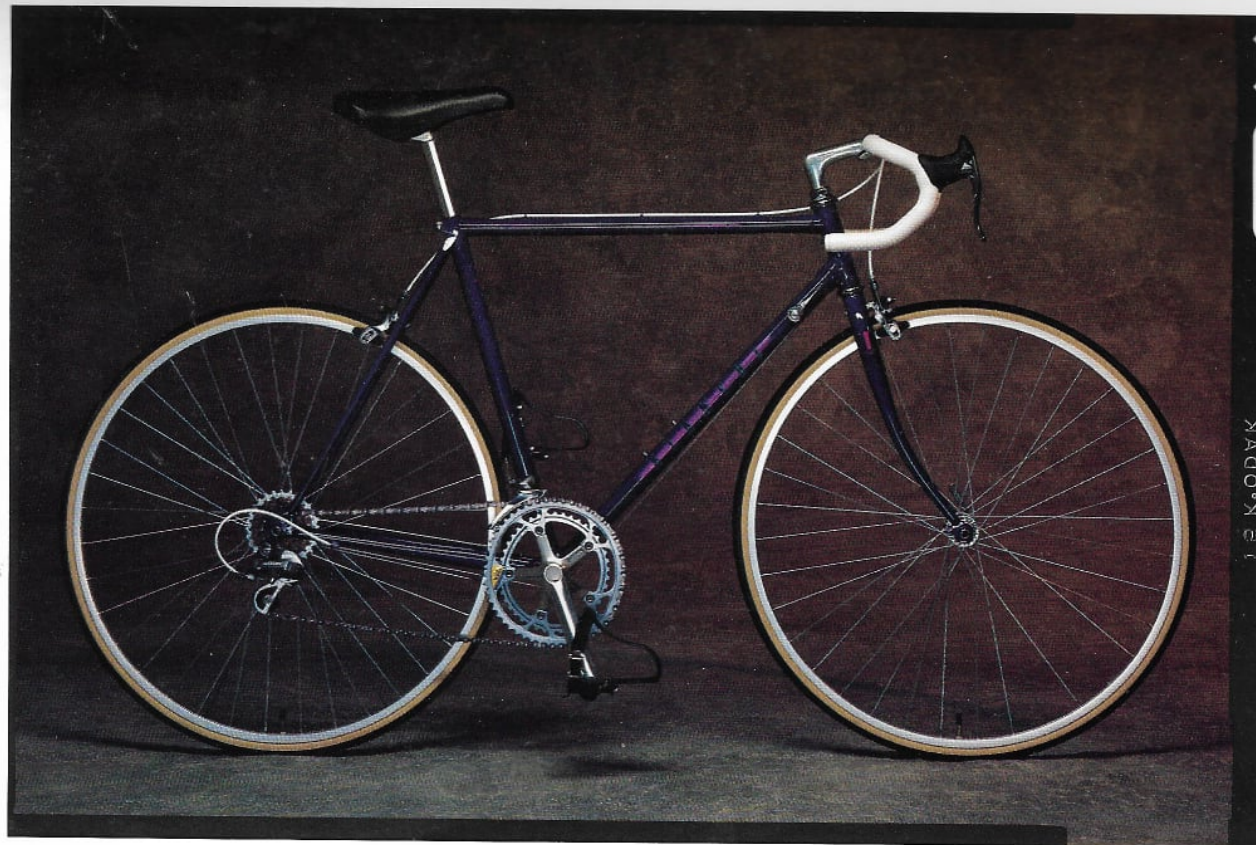
The Bianchi Forza. The Forza brings the design philosophy of Italy's greatest manufacturer to a Performance level road bike. With Tange double-butted chrome-moly frameset in our SuperSet 2 configuration, Shimano 14-speed Indexed Hyperglide shifting, Linear Response brakes.
