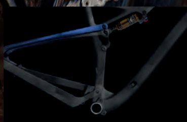
Total deflection of the swingarm requires less than 5kg of force on the saddle compared to 250kg required to fully compress the shock.
