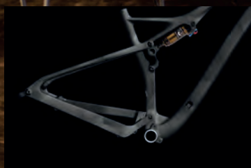
The swingarm flexes upward as the linkage moves
