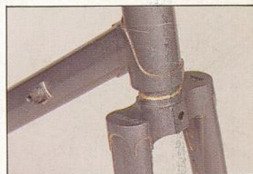
The bottom bracket, lugs, and fork crown are investment cast.
