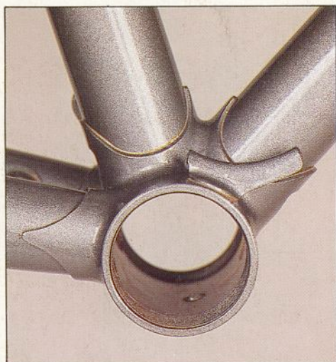
The bottom bracket, lugs, and fork crown are investment cast.
