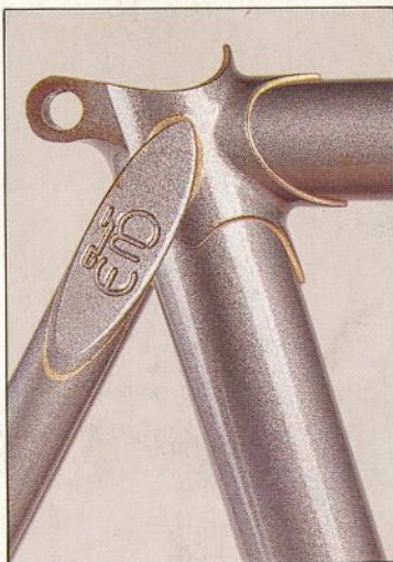
The bottom bracket, lugs, and fork crown are investment cast.
