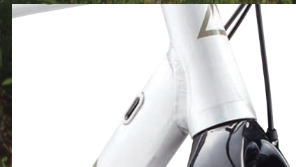
Internal Cable Routing
