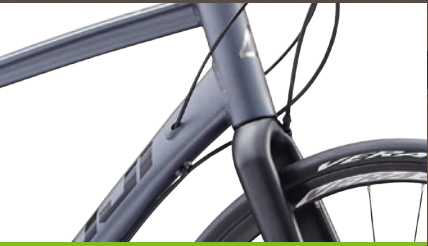
Internal cable routing across 1 series
