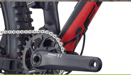
Internal Cable Routing
