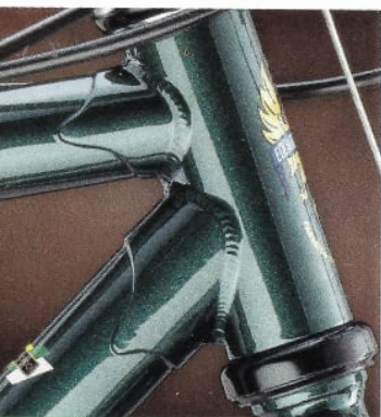
SuperLug's revolutionary design features "polycurve" lug points that are positioned laterally on the tubes.
