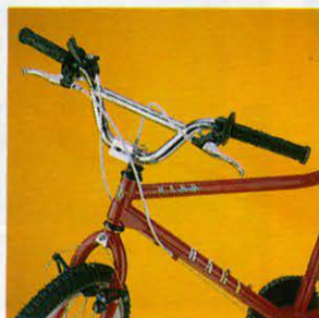
CONTROL CENTER The Rage's cross terrain bars, two finger levers, 6 speed shifter and Haro grips.
