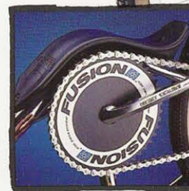
Sport: Odyssey Excalibur chromoly crankset. Fusion alloy Disc Drive sprocket. Replaceable high impact plastic bashguard.
