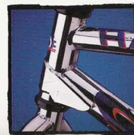
Group IC: 100% 4130 chromoly mainframe w/ wraparound head gusset.
