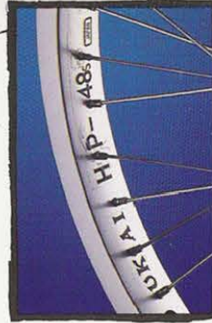
Master: Ukai HP-48 Equalizer 48 hole alloy rim. Stainless steel spokes.
