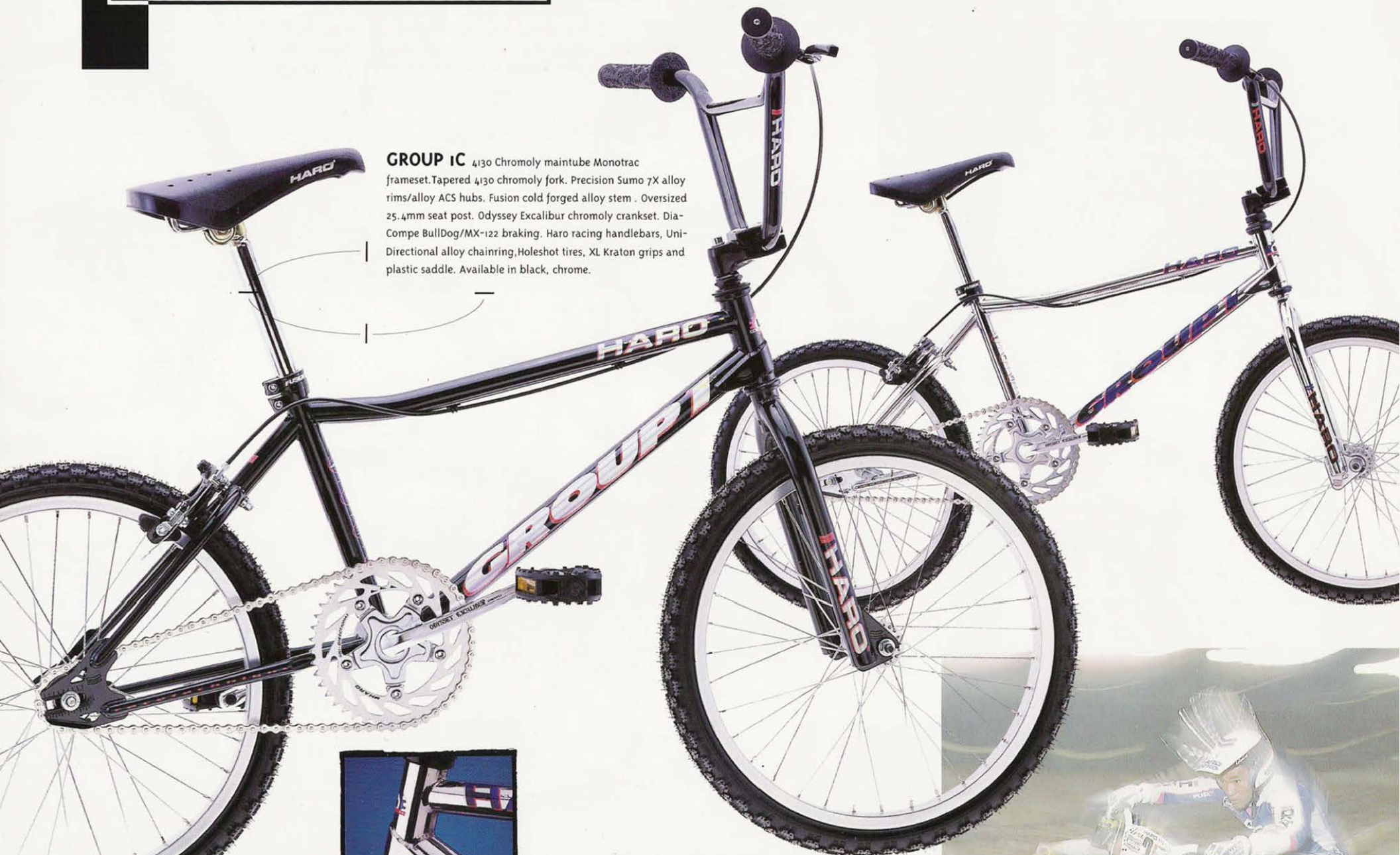
Group IC: 100% 4130 chromoly mainframe w/ wraparound head gusset.
