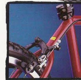
Group 1B: Fusion TwinTorc seat clamp. Oversize alloy micro adjust seat post. Dia-Compe Bulldog brake.
