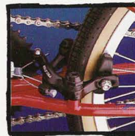
Edge: Rear U-brake. Sumo 48 hole alloy rim. Haro Multisurface tire.
