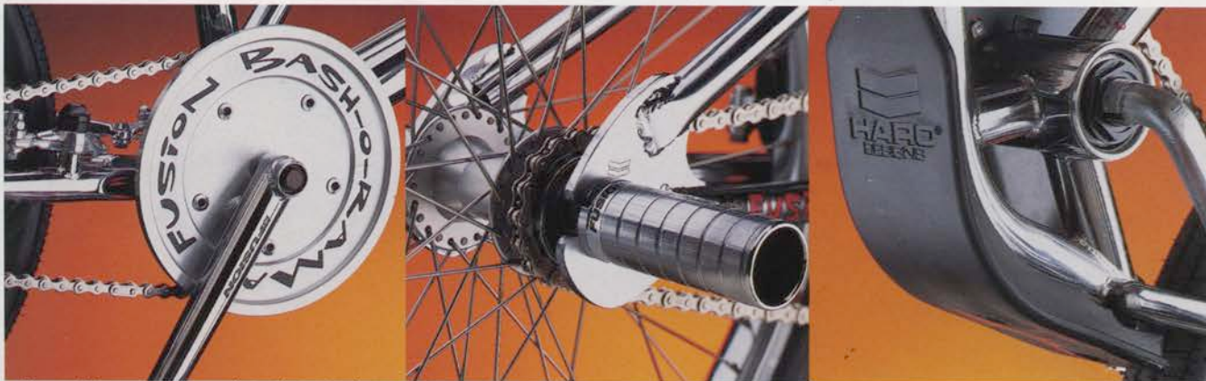
Blammo/Ultra: Fusion grind disk, Fusion 3-piece CRM0 crank, 990 U-brake.
