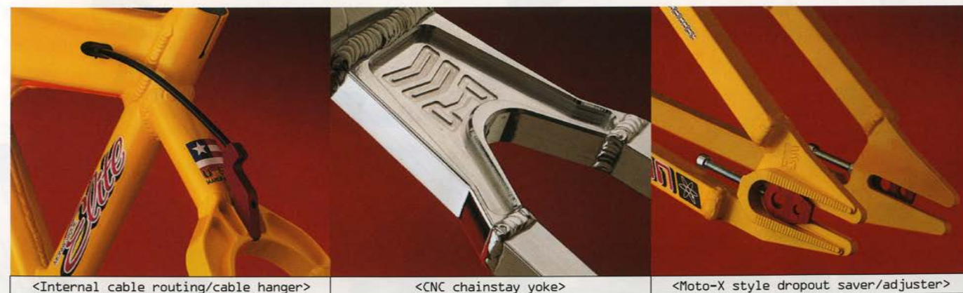
<Internal cable routing/cable hanger>
