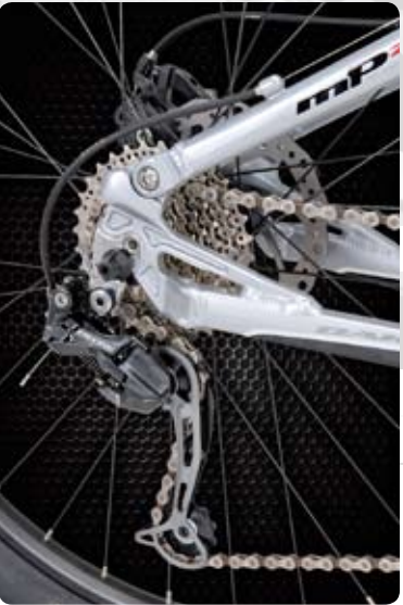
Both XC's offer Shimano's Shadow derailleur with a quiet, super low-profile design that won't slap the chainstay in rough riding conditions. Direct cable routing reduces the risk of housing snag. The Shadow also features a strong return spring that delivers positive, crisp shifts.
