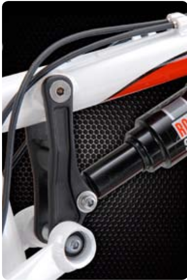
Dakar XC's mp2 suspension system is active with a near-vertical wheel axle travel path, plus excellent lateral & torsional stiffness for rear wheel tracking precision.
