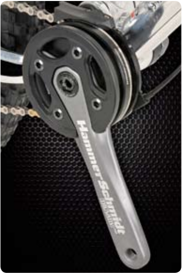
TruVativ's Hammerschmidt transmission technology is Truly Innovative! It's more than that. It's brilliant! Think of it as an internally geared hub in your bottom bracket shell, that eliminates your front derailleur and all of your chainrings 'cept one, without sacrificing gear range. You can now downshift in the front while you're drinking a beer without losing your chain or mis-shifting.
