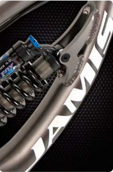
Our 10mm shock hardware is NOT the standard from our rear shock suppliers. We have to pay more for it and our production lead times are usually increased because we specify it. But the increase in lateral & torsional stiffness for our frames and the enhanced rear shock durability and performance is worth every extra dollar and every extra delivery day.
