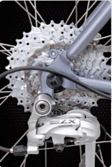
Every Coda offers a full complement of eyelets and rack mounts to simplify installation of a rear carrier and fenders.
