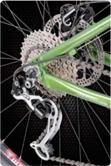
Shimano's new 12-36T HG61 cassette featured on Exile II is specifically designed to work with 29" wheels, offering a super low 36T gear that helps get these larger diameter wheels up hills as quickly as their 26" little brothers. But that new 12-36T cassette requires a new freehub to handle the higher torque generated by that larger diameter rear cog. Voila -- meet the new FH-M629 'niner specific rear hub!
