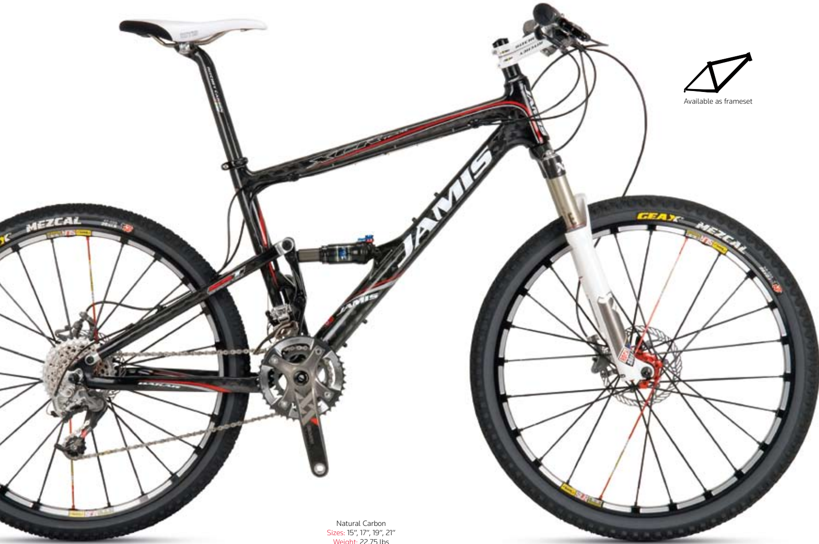
The revolutionary 2 x 10 drivetrain on the XCR Team is powered by a 42/28T TruVativ BB30 crankset that maximizes power transfer and stiffness while minimizing weight. The BB30 version we spec comes in at scant 694 grams! The chainrings are CNC-machined from 7075 alloy blanks that are 2mm thicker than the competition. That larger BCD and 2-piece insert-molded carbon construction deliver unparalleled stiffness. And Q-factor is a narrow 156mm!
