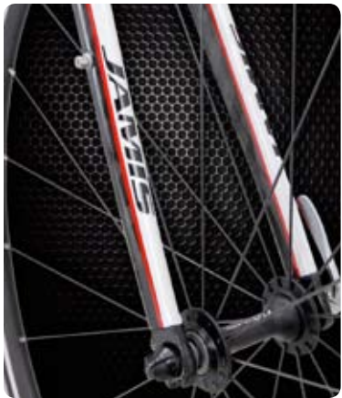
Allegro 4 & 3's full carbon composite fork is designed for lightweight steering precision. A perfect example of how we take all the knowlege we gain from designing and producing our award winning carbon competition road bikes and trickle that know-how down to provide top quality performance throughout the Jamis line-up.
