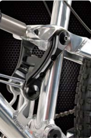
The XAM mp3 multi-link suspension design is optimized for strength and stiffness in the lightest weight package possible. Designed to offer superb pedaling efficiency with absolute downhill competency. It includes 10mm shock hardware for increased lateral & torsional stiffness and enhanced rear shock durability and performance.
