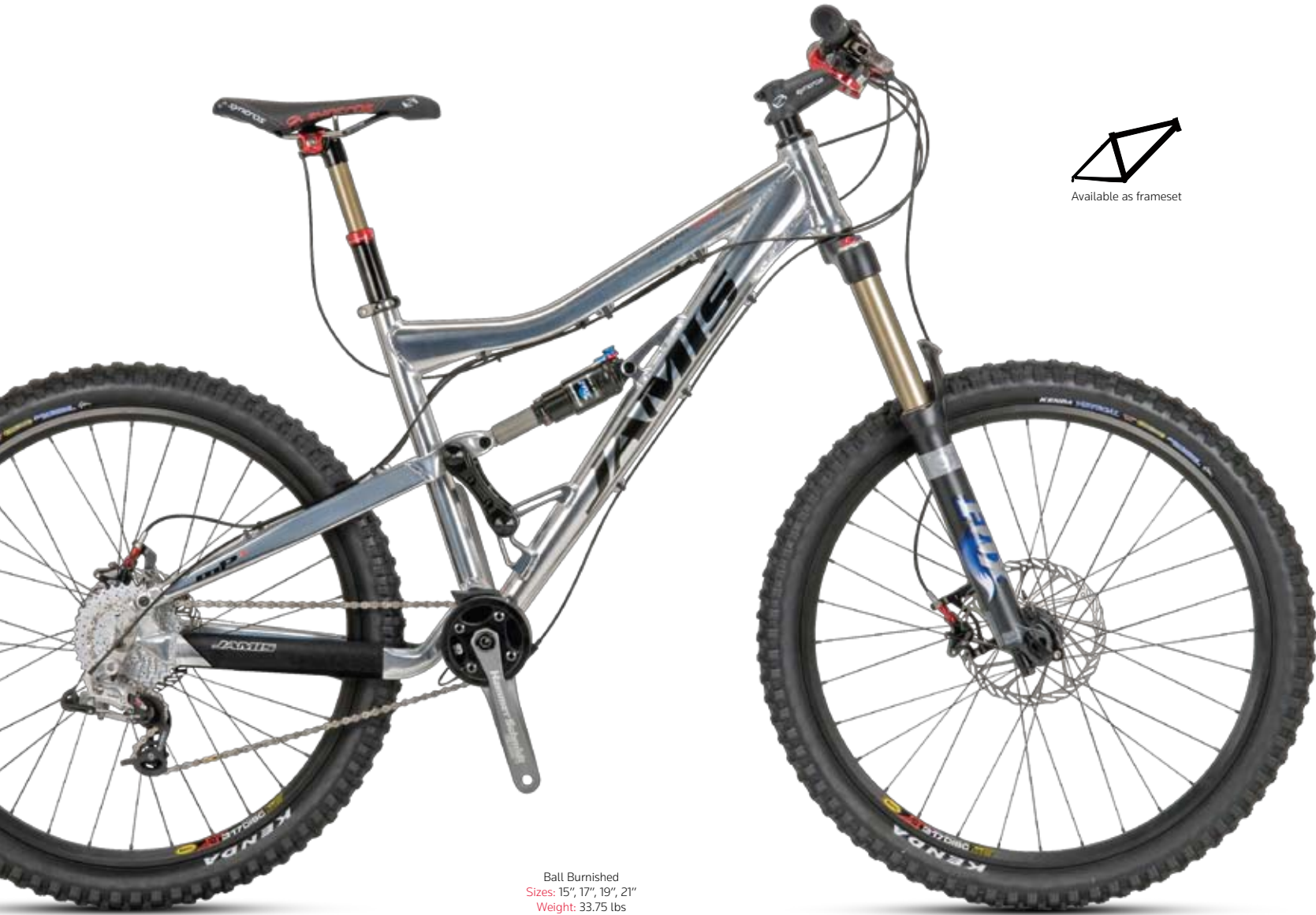
TruVativ's Hammerschmidt transmission technology is Truly Innovative! It's more than that. It's brilliant! Think of it as an internally geared hub in your bottom bracket shell, that eliminates your front derailleur and all of your chainrings 'cept one, without sacrificing gear range. You can now downshift in the front while you're drinking a beer without losing your chain or mis-shifting.
