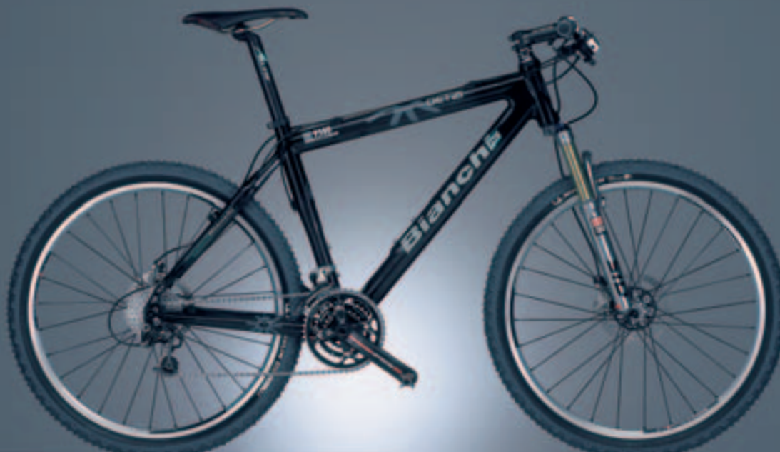
OETZI 9500 XL CARBON XTR/XT DISC, Y6B57, COLOUR EM - GROUP SHIMANO XTR/XT, FORK ROCKSHOX SID RACE, HANDLEBAR FSA XC-180 OS, STEM FSA OS150 LX SUPER OVER, SEATPOST SELCOF 91A CARBON, BRAKES SHIMANO XT DISC, CRANKSET FSA CARBON PRO TEAM ISSUE, WHEELS DT WIZARD XR4.1. ALSO AVAILABLE AS FRAMESET (X6B52).
