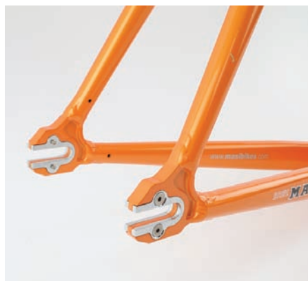
Masi 7005 T6 SL double butted aero tubed track frame w/ aero seat tube, rear wheel cutout & track dropouts w/ stainless steel inserts
