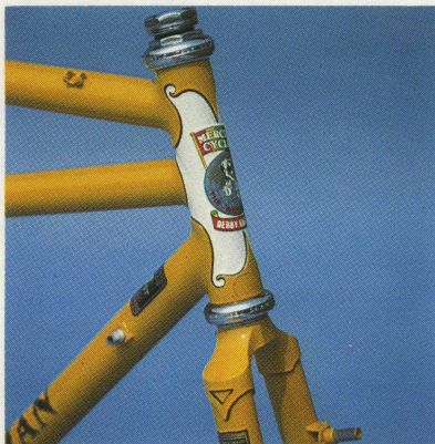
Hand cut Lugs on Mercian Tandems
