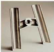
The brake bridge is precisely mitered before welding for a perfect fit. The center boss is machined from solid bar for rigidity.
