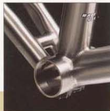
Merlin's signature "paddle weld" is a study in craftsmanship and strength.
