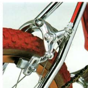
BRIDGESTONE's own patented SC (Self-Centering) brake with AW Brake Pads
