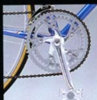
Chainwheel tapped for triple rings
