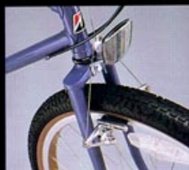
BRIDGESTONE 26 x 1.125 skinside Tire OFF/ON road pattern & SHIMANO AT-50 cantilever brake
