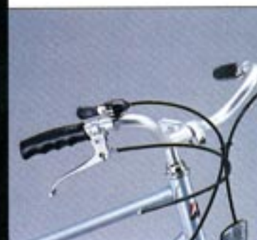
Thumb shifter with ratchet mounted on alloy handlebar
