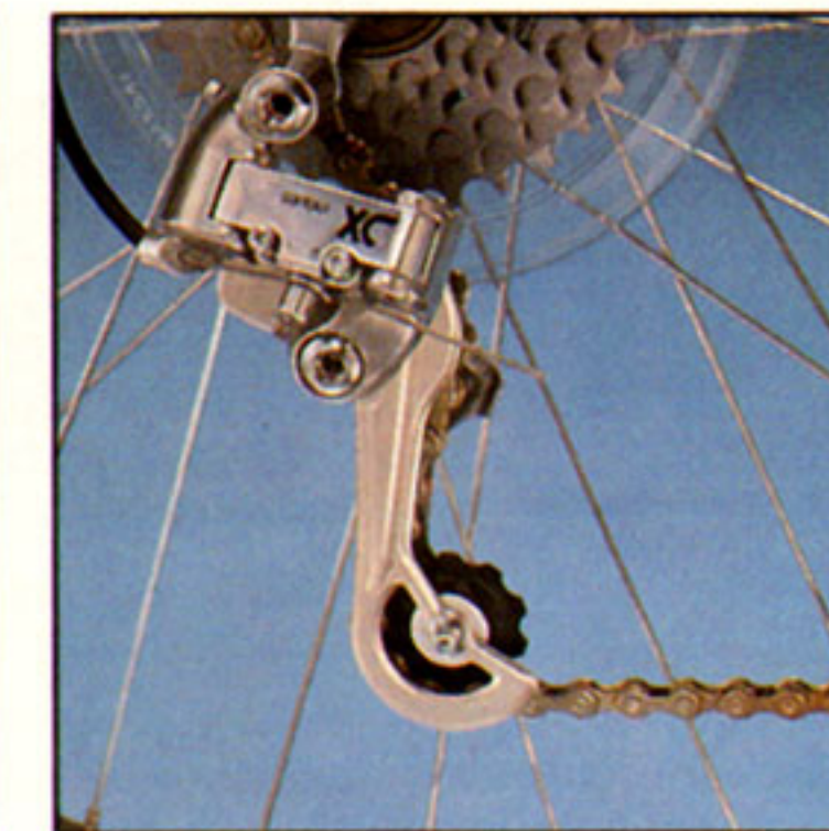
Suntour XC Series rear changer and New Winner 6-speed, 14-32, freewheel provide quick, responsive, wide range shifting.
