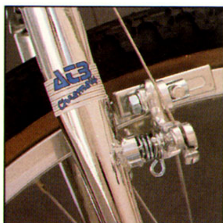
Chromoly forks and triple butted chromoly mainframe on all ATB™ models.
