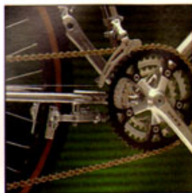
Suntour CB6100 roller cam brakes are positioned on the chainstay for greater braking efficiency.
