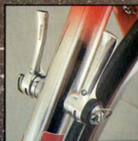
Shimano's Light Action SIS system ensure positive gear selection.
