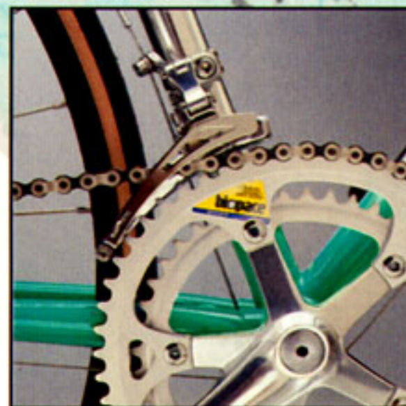
Shimano 105 cranks feature Biopace chainrings.
