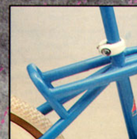
Kicktail standing platform is deep knurled for extra traction.
