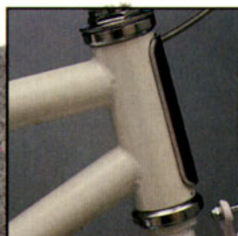
Heliarc welded 1 1/8" tubular chromoly means lightweight durability.
