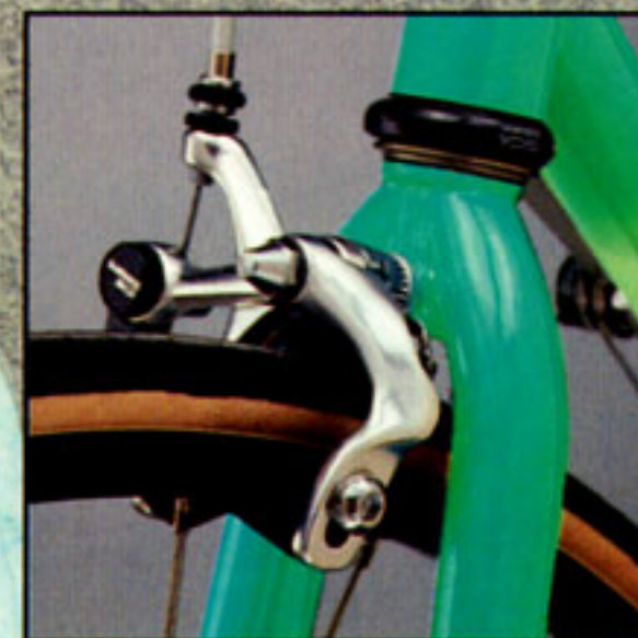
Aero Unicrown fork and Shimano 105 brake mean quick steering and stopping.
