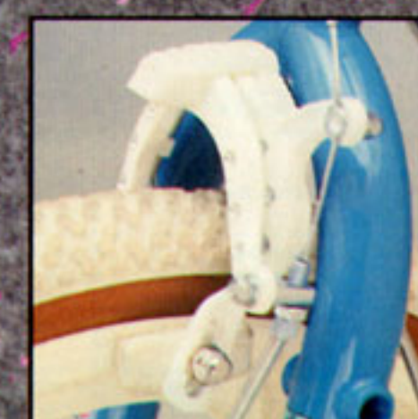
Brake has standing platform and recessed mounting nut.
