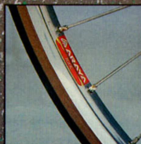
Araya 32 spoke alloy rim faced with stainless spokes.
