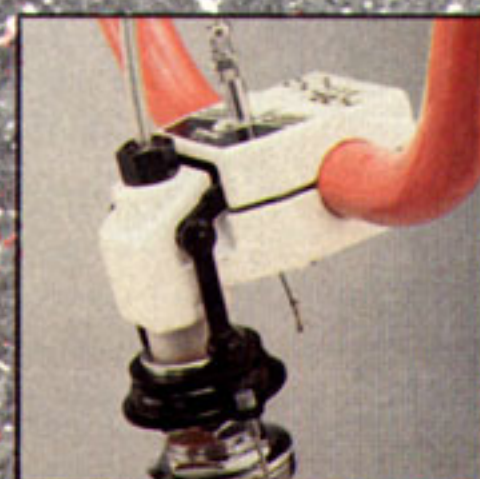
SR Spintech stem provides thru-the-stem cable routing.
