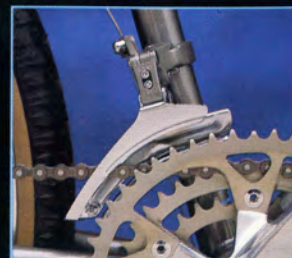
The new Exage Mountain front derailleur features SIS indexing or friction control shifting.
