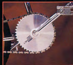
The heat treated Boron Steel cranks and Tioga CD alloy chainwheel.
