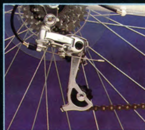
The SIS indexing derailleur system provides easy positive gear engagement.
