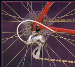
The Shimano derailleur system features positive SIS indexing gear selection.
