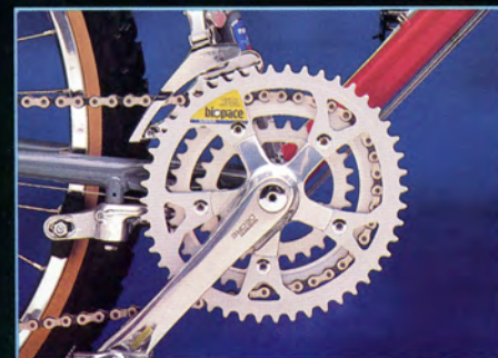
Shimano alloy crankset and Biopace chainrings provide maximum torque and energy transfer.
