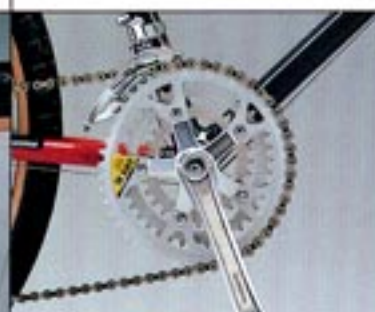
SHIMANO FC-B124 (Outer & center rings 600EX) chainwheel with BIOPACE rings
