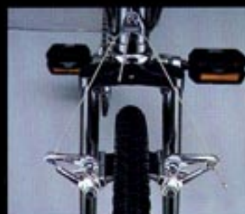
Oversize blades front fork & SHIMANO AT-50 cantilever brake
