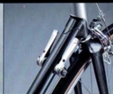
SUNTOUR New power shifter with ratchet mechanism
