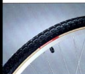
BRIDGESTONE 26 x 1.4 tire & ARAYA 7S alloy rim
