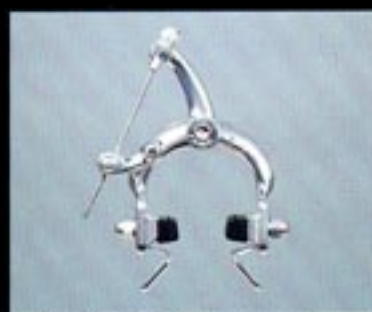
BRIDGESTONE Self-Centering brake with tire guides
