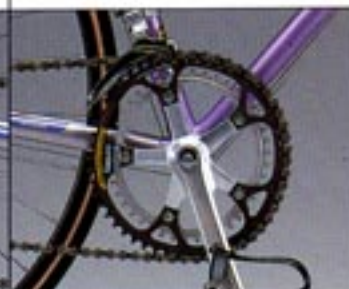
SHIMANO N600EX chainwheel with hard anodized BIOPACE rings & front derailleur
