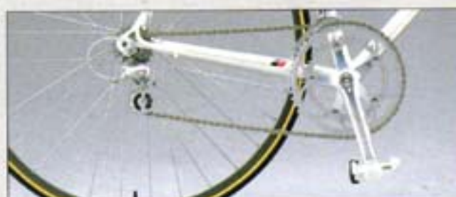
53 x 39T chainring and 12 - 20T rear sprocket and LOOK pedal
