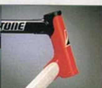
Originally designed lost-wax head lug (upper and lower)
