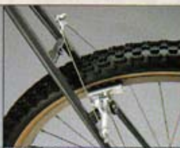
RITCHEY FORCE tire on ARAYA RM-20 super hard rim and DIA-COMPE #982 cantilever brake
