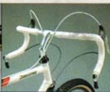
Newly-designed drop handle for Mountain Bike and SUNTOUR bar-end shifter
