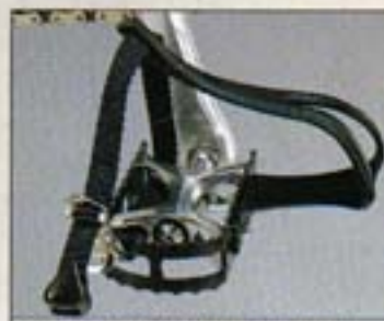
SUNTOUR XC-COMPE pedal with clip and strap
