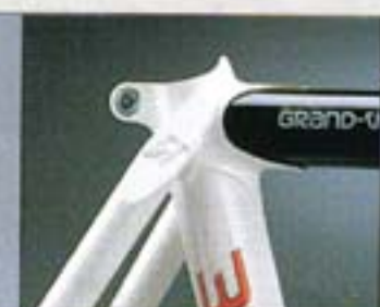
Originally designed lost-wax seat lug and seatstay cap
