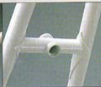
Reinforced seatstay bridge and brake boss for recessed anchor bolt
