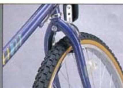
Tig welded Uni-crown
