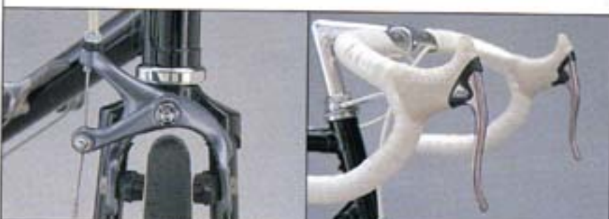
SHIMANO EXAGE-Action SLR brake/aero lever
