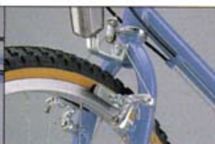
Cantilever brake on Tig welded Uni-crown
