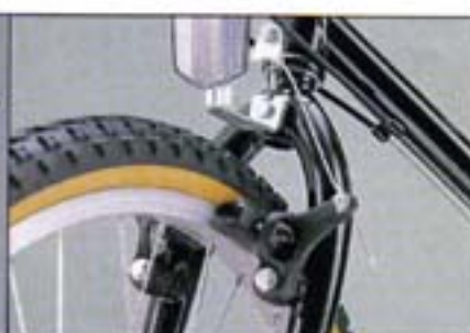
EXAGE-Country SLR cantilever brake
