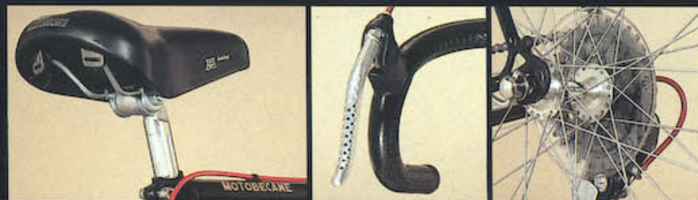
1 - ANATOMIQUE PADDED SEAT WITH CTP 6 MICRO ADJUSTER SEAT POST, BRAZED-ON CABLE GUIDES. - 2 - WEINMANN DRILLED LEVERS WITH MOTOBECANE HANDLEBAR SLEEVES. - 3 - MAILLARD ALLOY QUICK RELEASE, REAR HUB WITH HELICOMATIC CLUSTER AND SEDISPORT CHAIN.
