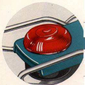
New Electric 360° Flashing Dome Warning Signal.
