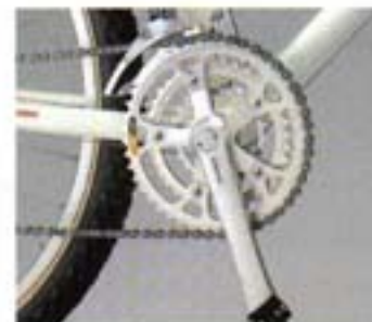
Deore XT crank has shorter than normal BB spindle, for lower Q factor.
