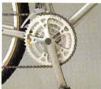
Shimano 500LX crank has round alloy rings for smooth pedaling and minimal weight.
