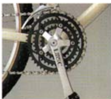
Ritchey crank is elegant, strong, and has a low Q factor.
