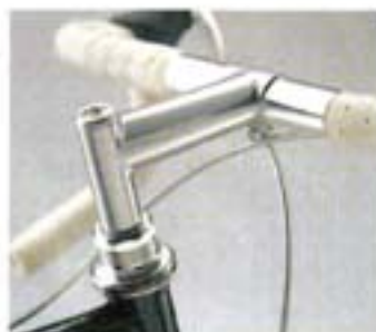
Eighty degree Ritchey stem has more range of height than standard stem, weighs 25% less, and won't ever creak.
