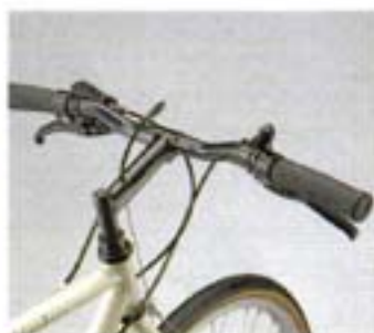
Ninety degree stem positions bars correctly for athletic street riding.
