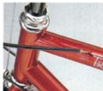
Slotted cable stops cut cable-servicing time by 90%.
