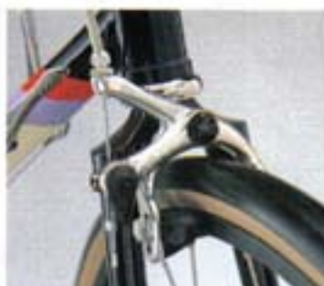
Dia-Compe sidepulls have preferred single-pivot design, and are cold-forged, for strength.
