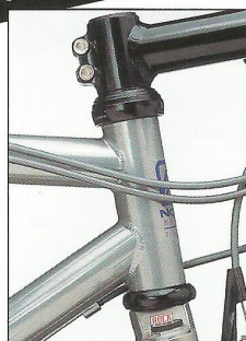
Dia-Compe "Ahead" system. Simple, clean, ultra light.
