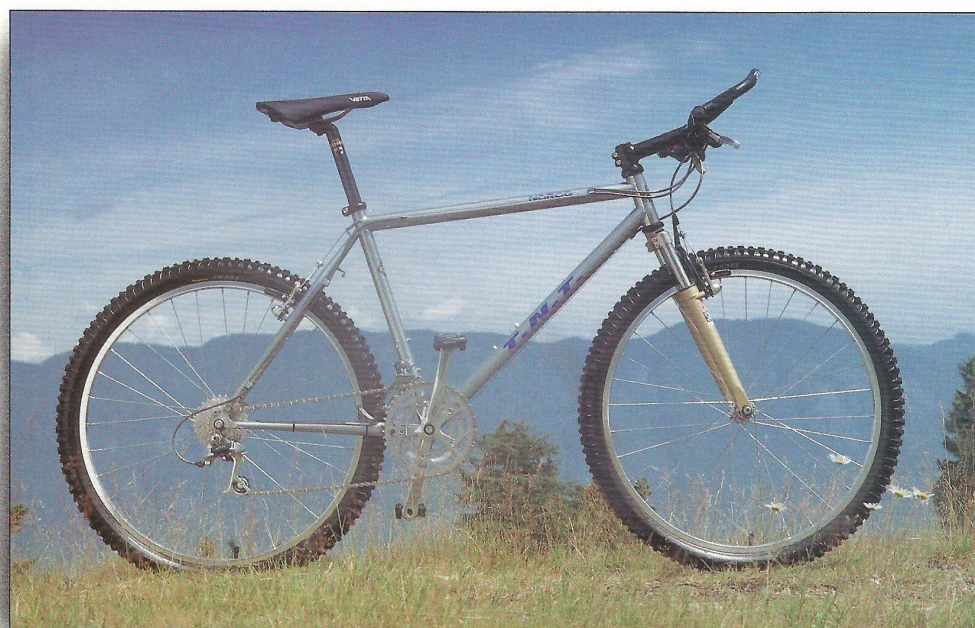
Dia-Compe "Ahead" system. Simple, clean, ultra light.
