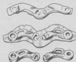
TOP: AFTER THE FIRST STOMPING. MIDDLE: AFTER THE SECOND STOMPING, SHOWING EXCESS. BOTTOM: EXCESS REMOVED, READY FOR FINISHING.
