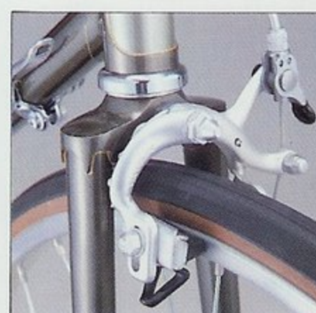
Dia-Compe G500N alloy side-pull with quick release and tire guides.
