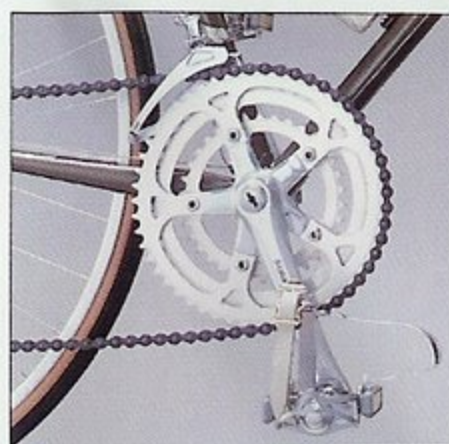
Sugino TGT forged alloy triple crankset and KKT Top-Run alloy quill pedals with toe clips and
