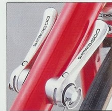
Shimano New 600 EX down tube brazed on shift levers.
