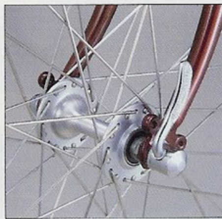
Semi-Large sealed bearing hub with quick release.
