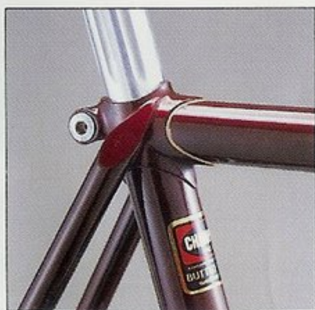
Lostwax seat lug and semi wrap-seat stay.
