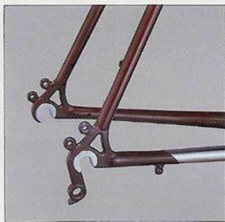
Forged vertical drop out forkends with dual eyelet.
