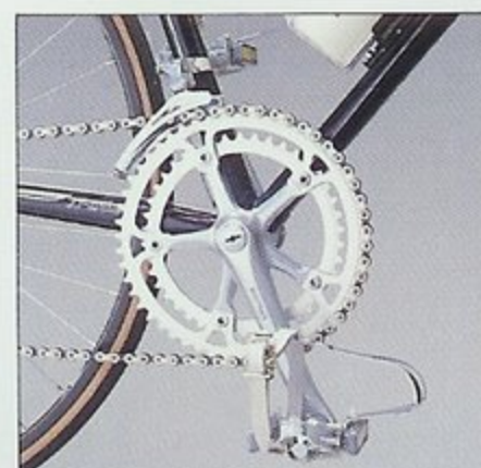
Sugino AS forged alloy crank set and KKT Pro Vic II pedal with toe clips and straps.
