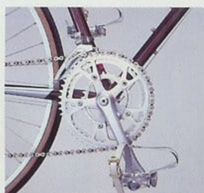
Shimano Biopace 50/44/28T crank set, Shimano Deore XT GS front derailleur and KKT Pro-Vic II A pedals with toe clips and straps.
