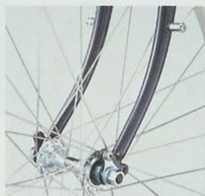
Brazed on front carrier studs and Suzue MTB-SS sealed mechanism hub.
