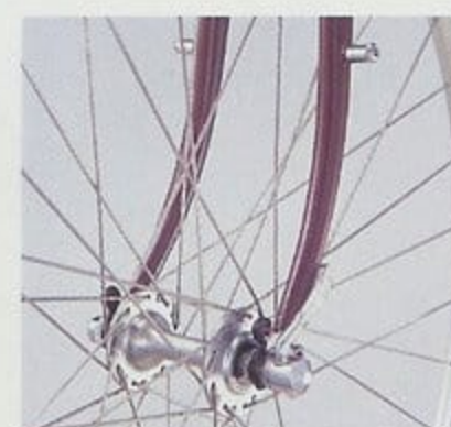
Brazed on front carrier studs and Sanshin Gyromaster sealed bearing hub.
