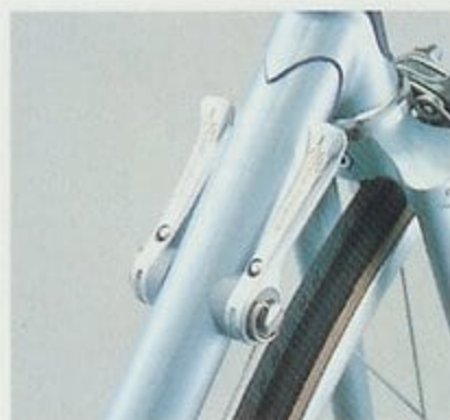
Shimano 105 down tube brazed on shift levers.
