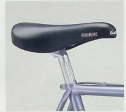
Selle Italia Turbo saddle. Shimano New Dura-Ace EX seat post, Columbus SP/SL frame and lostwax seat lug.
