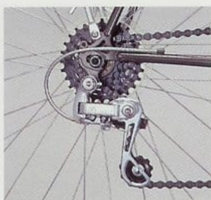
Shimano AL-11 rear derailleur and shimano UG 5-speed freewheel.
