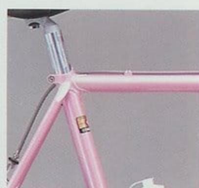
Columbus SP/SL frame, lostwax seat lug and Campagnolo seat post.
