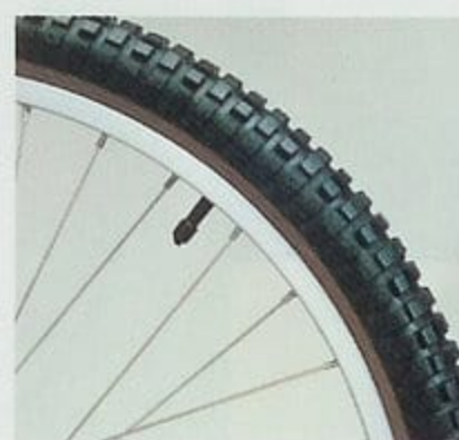
26" X 1.75" alloy rim and 26" X 2.125" open side tire.
