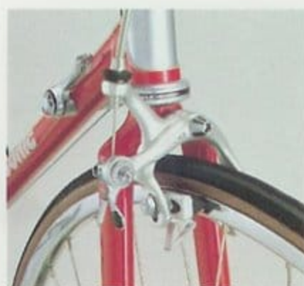
Tange C-2 sloping crown and Shimano New 600 EX brake arch
