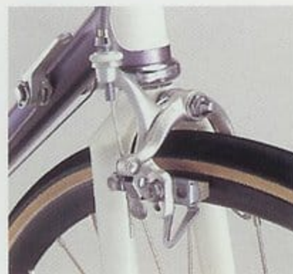
Tange Cr-Mo fork, C-2 fork crown and Campagnolo Victory brake arch.
