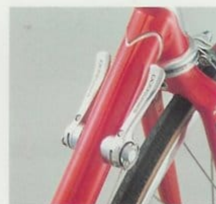
Shimano New 600 EX down tube brazed on shift levers.
