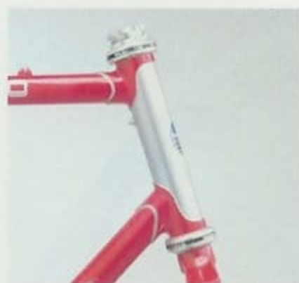
Italian cut head lug with Shimano New 600 EX head set and pump peg.
