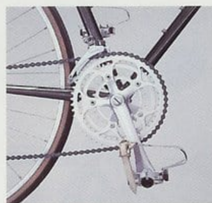
Shimano ART 50/42/28T crank set, Shimano AL-11 front derailleur and KKT Provic IIB pedals with toe clips and straps.
