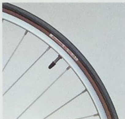
Araya 20A, 700C narrow alloy rim and Panasonic 700 X 25C Racing Extra 100 PSI
