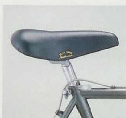
Selle Italia 0423 anatomic saddle with SR CT-P5 250mm long seat post and fastback seat stay end
