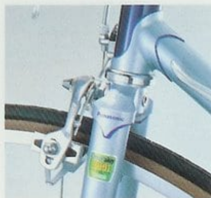
Shimano Z570 side-pull brakes with tire guides and recessed mounting bolt.
