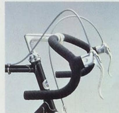
Nitto Model 155 alloy handlebar and Nitto Pearl 10 alloy stem
