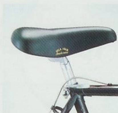
Selle Italia 0451A anatomic saddle with SR CT-P5 250mm long seat post and quick release seat binder bolt set.
