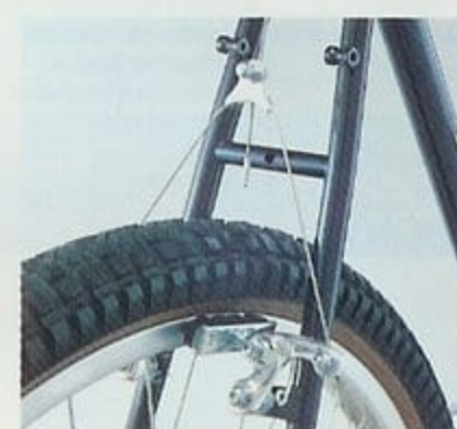
Brazed on rear carrier studs and Dia-Compe No.981 cantilever brakes
