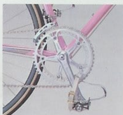
Campagnolo Super Record 1409/A crank set, front derailleur and 1037/A pedals with toe clips and straps.
