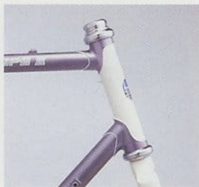
Lostwax head lug with Campagnolo Victory head set and pump peg.
