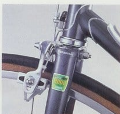
Shimano Z570 side-pull with tire guides.
