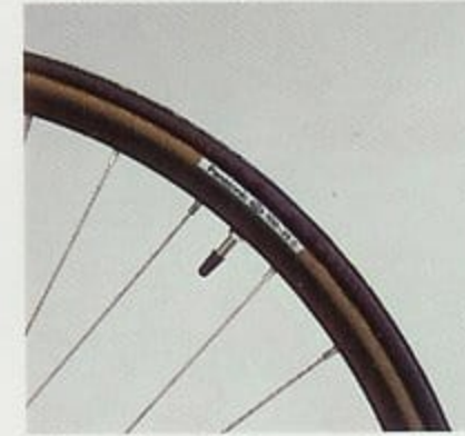
Araya 20A, 700C, alloy black anodized rim and Panasonic 700 X 25C open side 100PSI tire.
