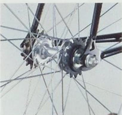
Alloy hub with 16T freewheel and 15T fixed sprocket, forged rear ends.
