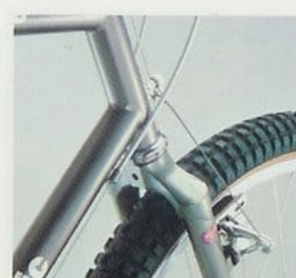
Tange Cr-Mo double butted tig welding frame and Tange MT-4 fork crown.
