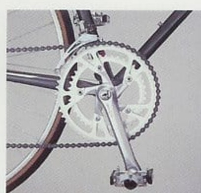
SR CRC-301 alloy crank set and KKT Pro-Vic II B Pedals.
