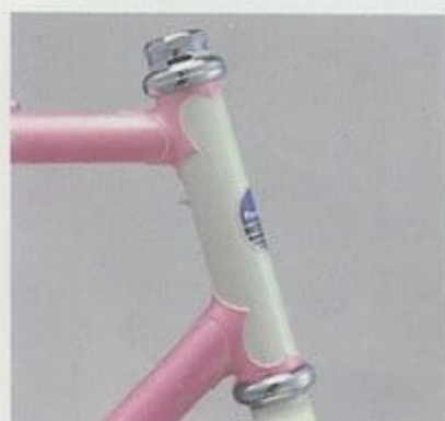
Lostwax head lug with Campagnolo Nuovo Record head set and pump peg.
