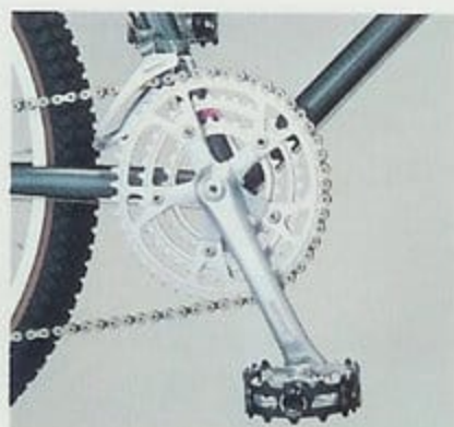
Shimano New 600 EX Biopace crank set, Shimano Deore XT and Sun Tour PL-5100 XC-II pedals
