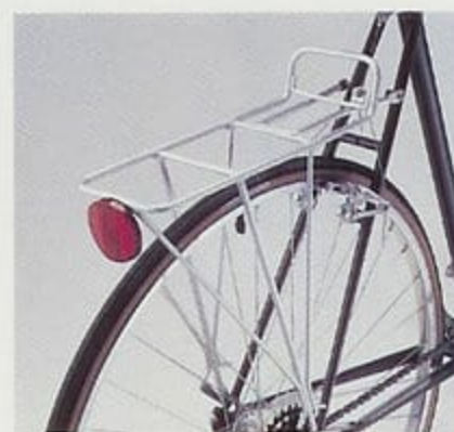
Alloy rear carrier and Shimano AT-50 cantilever brakes
