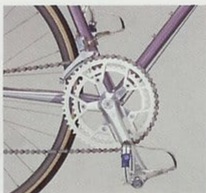
Campagnolo Victory crank set, front derailleur and pedals with toe clips and straps.
