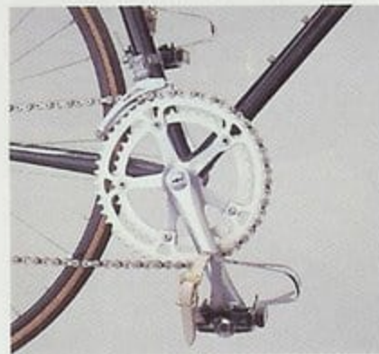
Sugino ALP forged alloy crank set and KKT Pro-Vic II B Black pedals with toe clips and straps.
