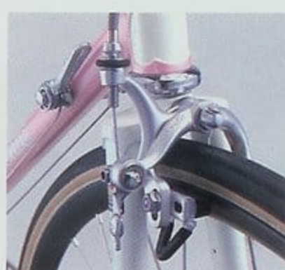
Columbus SP front fork, Tange C-10 lostwax fork crown and Campagnolo Super Record brake arch.
