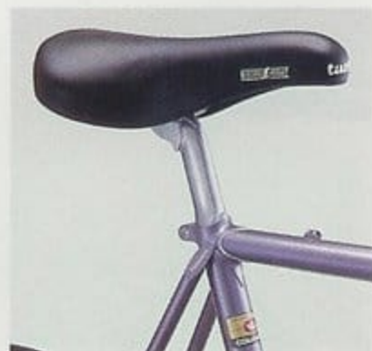
Selle Italia Turbo saddle, Campagnolo seat post and Columbus SP/SL frame
