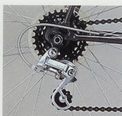
Shimano L513 rear derailleur and Shimano 6 speed freewheel.
