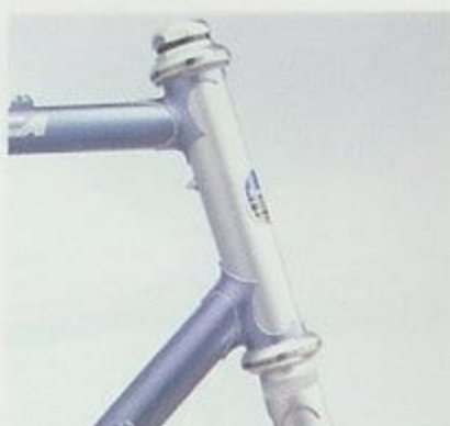
Lostwax head lug with Shimano New Dura-Ace head set and pump peg.
