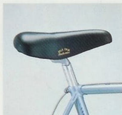
Selle Italia 0451A anatomic saddle with SR CT-P5E micro adjusting seat post and Lostwax seat lug.
