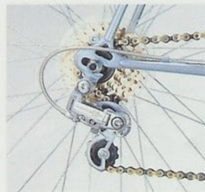
Shimano 105 rear derailleur and Shimano UG gold 6 speed freewheel.
