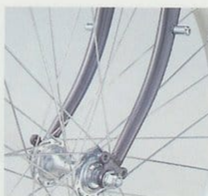
Sun Tour. Sealed bearing hub and brazed on front carrier studs
