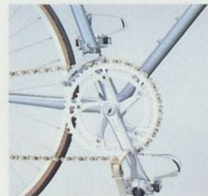
SR CRC-101 alloy crank set and KKT Pro-Vic II B pedal with toe clips and straps.
