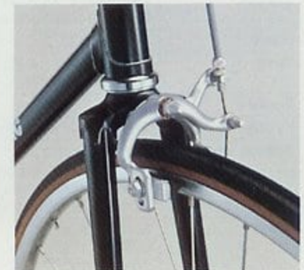
Dia-Campe 500 alloy side-pull brake.
