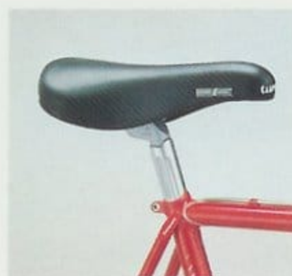
Selle Italia Turbo saddle with SR CT-P5 micro adjusting seat post and Lostwax seat lug.
