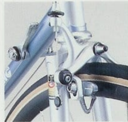
Columbus SP front fork, Tange C-10 lostwax fork crown and Shimano New Dura-Ace EX brake arch
