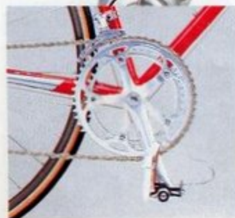
SunTour Superbe Pro crankset, front derailleur and sealed bearing pedals with toe clips and straps.
