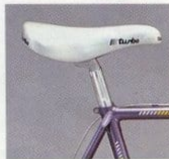
Tange champion No.1 frame, lostwax seat lug and SR CT-P5 micro adjusting seat post.
