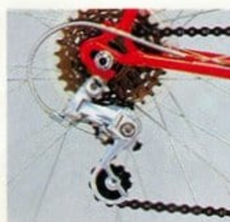
Shimano L523 SS rear derailleur and Shimano Z012 6-speed 14-28T freewheel.
