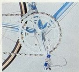
Campagnolo Victory crankset, front derailleur and pedals with toe clips and straps.
