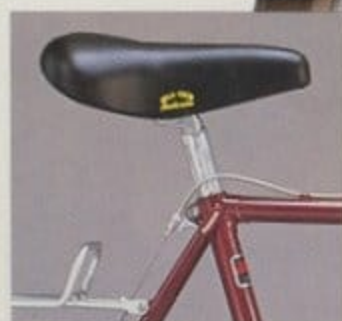
Selle Italia 0422-V anatomic saddle and SR CT-P5E micro adjusting seat post.
