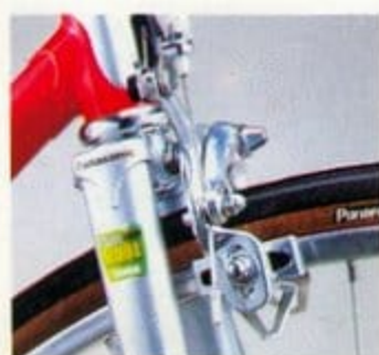
Shimano Z570 side-pull with Q.R., guide brake arch and Tange Mangalay front fork.
