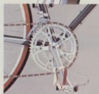
Shimano Biopace crankset, Shimano Deore XT Super Plate rear derailleur and Shimano 600UG silver 6-speed freewheel. Road pedal with toe clips and straps.
