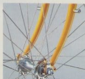
SunTour XC sealed bearing hub and brazed on front carrier studs.
