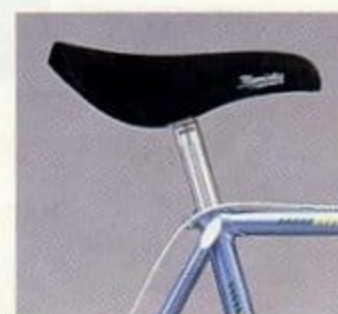
Selle Italia Mundialita saddle with Sugino SP-KCL micro adjusting seat post.
