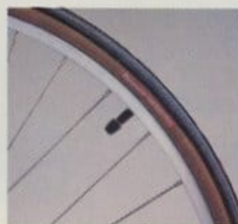
Araya 16A [3] 27" x 1 1/4" alloy rim and Panaracer 27" x 1 1/4" Tour Guard with Kevlar belt 90PSI tire.
