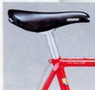
Columbus SP/SL frame and lostwax seat lug, Selle Italia Turbo saddle with SunTour Superbe Pro seat post.
