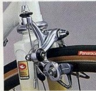
Columbus SP front fork, Tange C-10 lostwax fork crown and Shimano New Dura-Ace brake arch.
