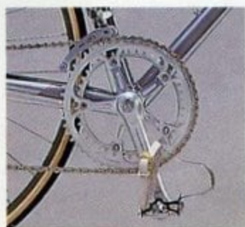
Campagnolo Super Record 1049/A crankset, front derailleur and Record 1037/A pedals with toe clips and straps.
