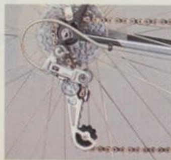
Shimano Deore XT Super Plate rear derailleur and Shimano 600UG silver 6-speed freewheel.
