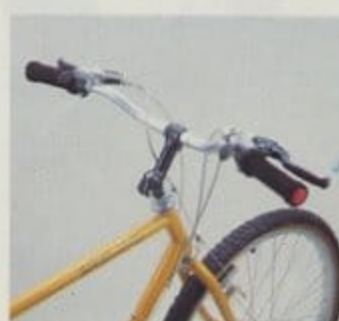
Nitto B801AA-F handlebar, Nitto MT-2 black handlebar stem and SunTour XC-Sport power brake levers.
