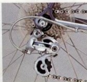
Shimano New 600 EX S.I.S. rear derailleur and 6-speed freewheel.
