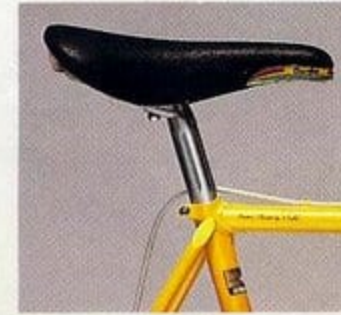
Columbus SP/SL frame, lostwax seat lug and Selle Italia Super Turbo saddle with Shimano New Dura-Ace seat post.
