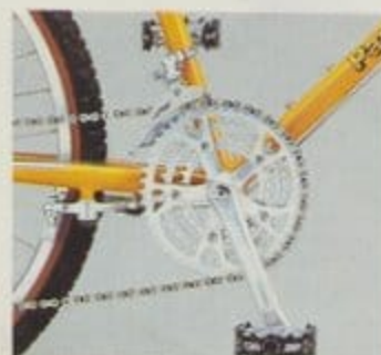
Shimano Biopace crankset, SunTour XC front derailleur and SunTour XC pedals.
