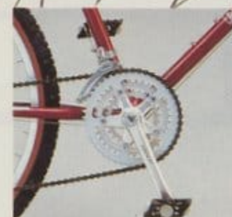
Sugino TGT crankset, Shimano AL-11 front and rear derailleurs, Shimano MX-15 black pedals.
