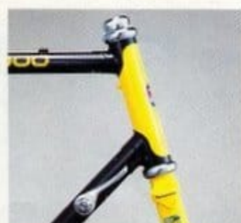
Italian cut head lug with Tange SE2S sealed mechanism headset and brazed on pump peg.
