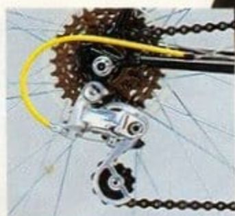
Shimano L525 SS S.I.S. (Shimano Index System) rear derailleur and Shimano Z12 6-speed freewheel.
