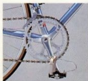
Sugino GLP special crankset, SunTour Sprint front derailleur and KKT Pro-Vic II B black pedals with toe clips and straps.
