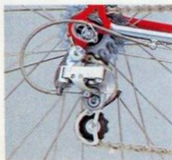
SunTour Superbe Pro rear derailleur and SunTour New winner 7-speed freewheel.
