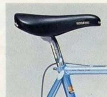
Columbus SP/SL frame and lostwax seat lug, Selle Italia Turbo saddle with Campagnolo Victory seat post.
