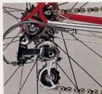
Shimano New Dura-Ace rear derailleur and 6-speed freewheel.
