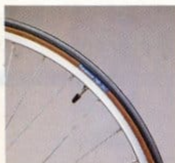
Araya 20A, 700C narrow alloy rim and Panaracer 700 X 25C Racing Extra 100PSI tire.
