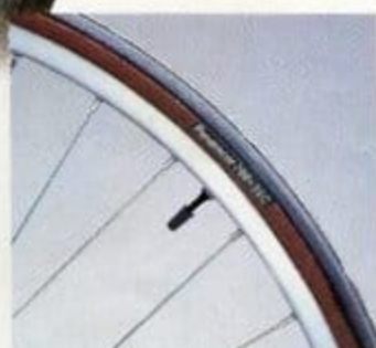
Ukai 20A 700C alloy rim and Panaracer 700 X 25C open side 100PSI tire.
