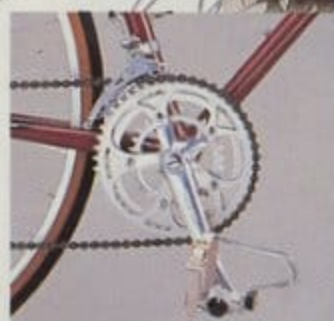
Shimano ART crankset, Shimano Z012 5-speed 14-28T freewheel and KKT Pro Vic II B pedals with toe clips and straps.
