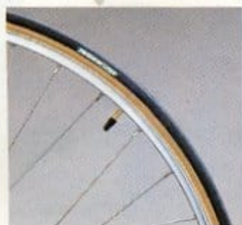
Araya 16B alloy tubular rim and Panaracer tubular 230gr. Leger tire.
