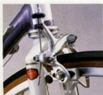
Tange C-2 sloping fork crown and Shimano New 600 EX brake arch.
