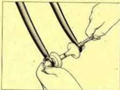
With the lever sticking straight out, screw the opposing cone in until it stops and there are no gaps between the dropouts and Q/R.
