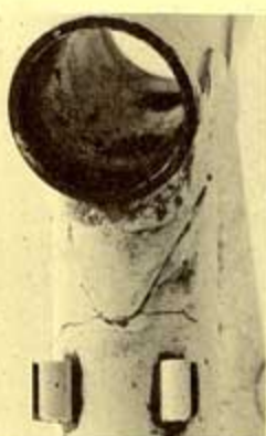
A "can-opener" break underneath the down tube. Next time, a thinner lug with a rounder tip? Fatigue.
