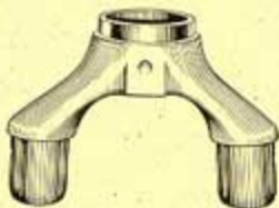
A modern, investment-cast version of the crown pictured at left. No filing needed — one reason builders like cast crowns.
