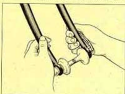
It requires firm pressure to close the lever securely and completely. Note the grip and the finished lever position. Do it right!
