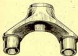
The original Cinelli (Italian). Forged, strong, and crude, it required much filing to lighten and beautify. No longer made.
