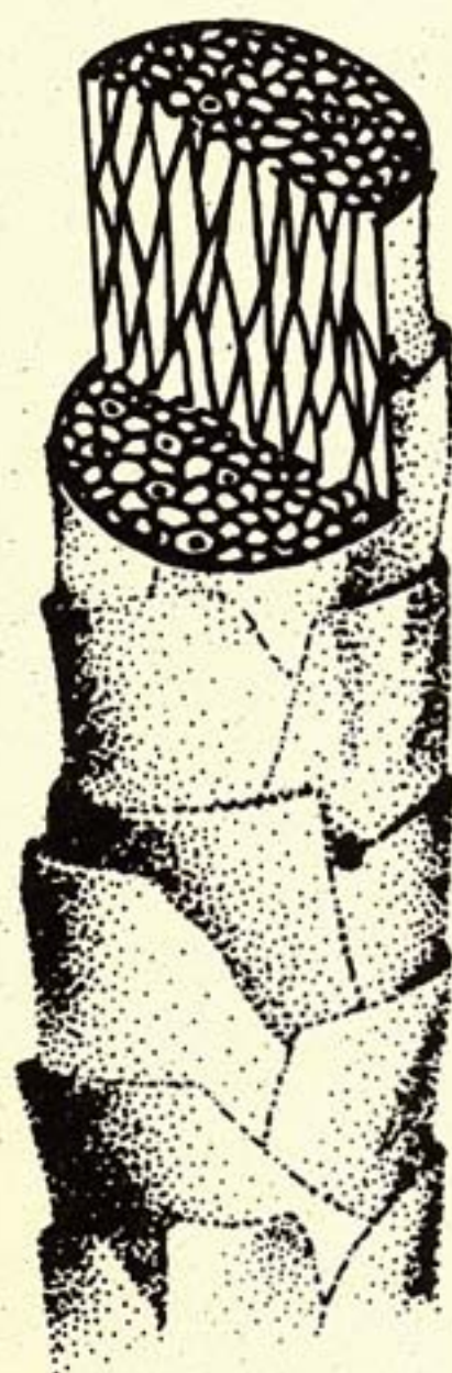
A WOOL FIBER HAS OVERLAPPING SCALES THAT TRAP DIRT NEAR THE SURFACE, WHERE IT IS EASILY WASHED OUT.
