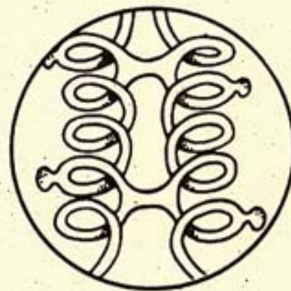
EACH WOOL FIBER HAS A SPIRALING CRIMP WHICH LETS IT STRETCH, THEN SPRING BACK.
