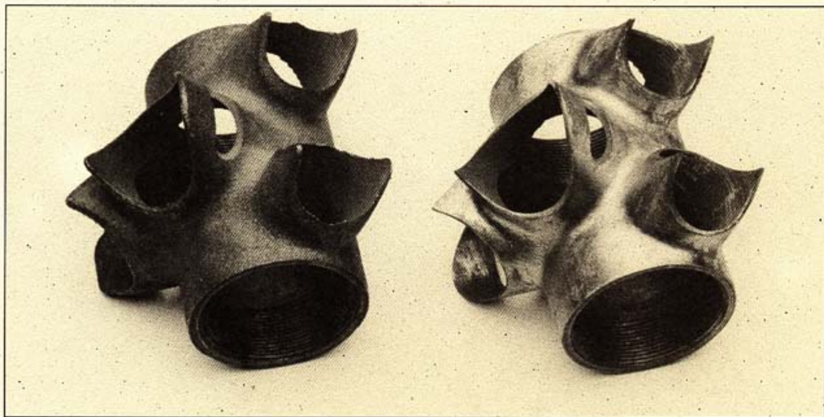
FISCHER BOTTOM BRACKET SHELL (MASI STYLE, FROM 1973) READY FOR FILING
