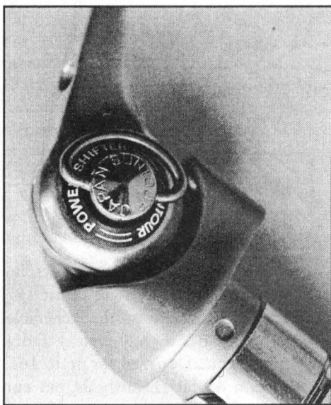
Step 6: Put the plastic SunTour badge back on (if it fell off), and then hold it all together with the wing bolt. These are the smoothest, slickest, best bar-end shifters you can get.
