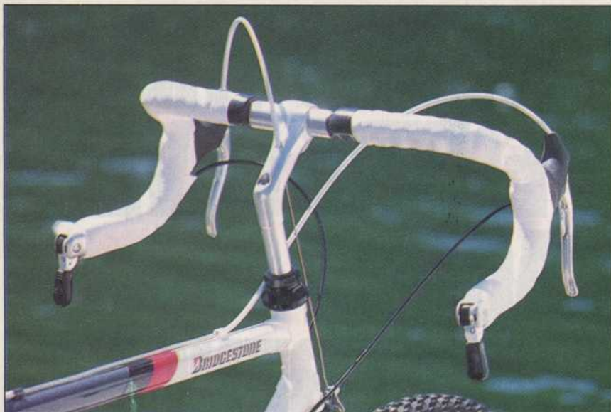
Slightly flared, heat-treated drop bars on the Bridgestone MB-1 aid comfort, control, and climbing efficiency.
